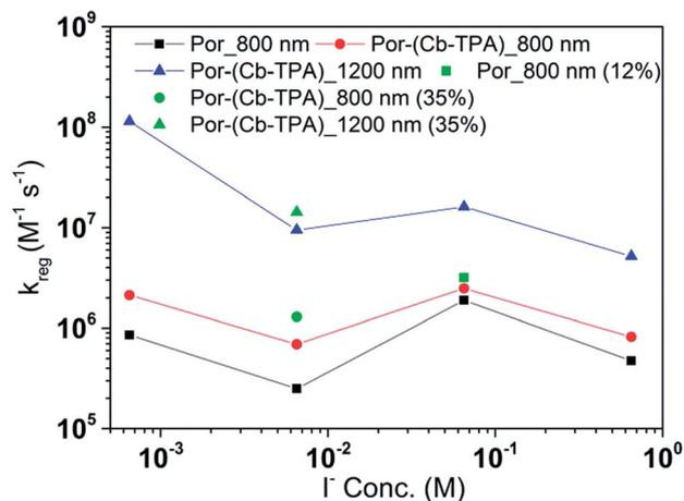
Fig. 8 Regeneration rate constant of Por and Por-(Cb-TPA) versus the concentration of  $I^-$ . Por with 12% dye-loading probed at 800 nm and Por-(Cb-TPA) with 35% dye-loading probed at 800 nm and 1200 nm are also shown.
