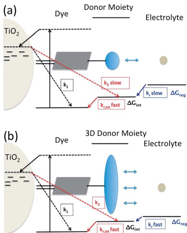
Fig. 1 Utilization of intramolecular hole transfer to enhance dye cation regeneration. (a) Reduced recombination and slower regeneration kinetics; (b) faster dye regeneration kinetics at a smaller driving force using a tridimensional donor moiety.
