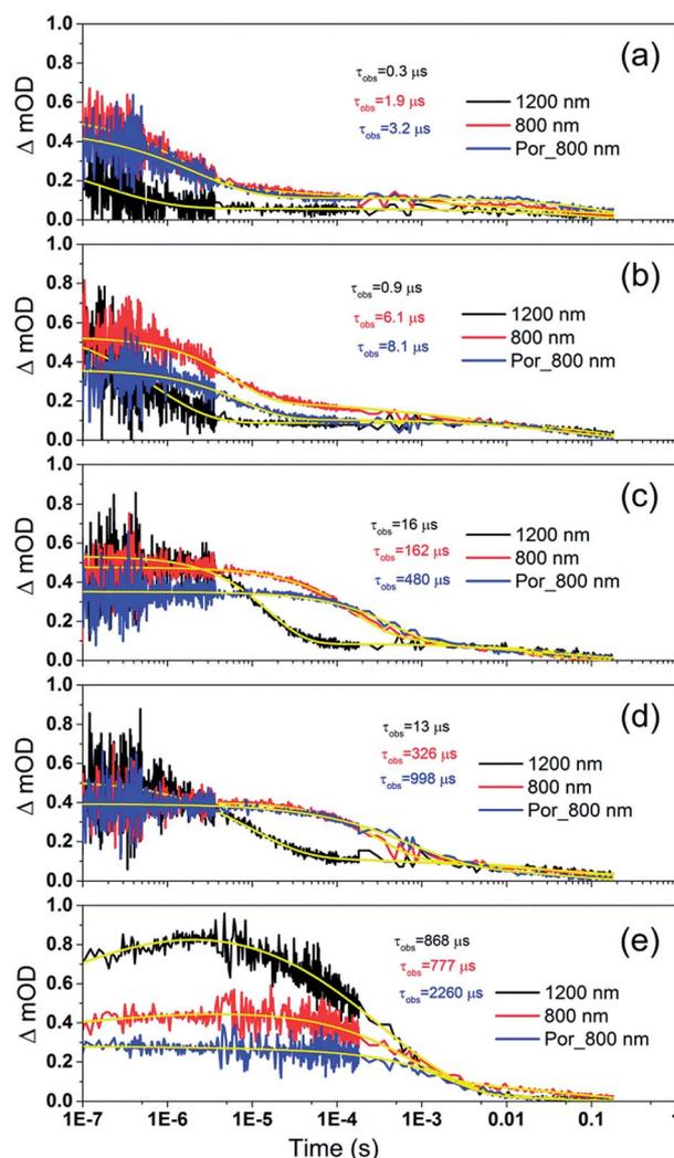
Fig. 7 Transient absorption decay and fitted curves of  $\text{TiO}_2\text{-Por-(Cb-TPA)}$  probed at 1200 nm (black) and 800 nm (red) and  $\text{TiO}_2\text{-Por}$  probed at 800 nm (blue) with five  $\text{I}^-/\text{I}_3^-$  electrolytes after pulsed 532 nm laser irradiation. (a)  $\text{I}_1$ , (b)  $\text{I}_0.1$ , (c)  $\text{I}_0.01$ , (d)  $\text{I}_0.001$  and (e)  $\text{I}_0$  (532 nm, 45–50  $\mu\text{J cm}^{-2}$  per pulse; repetition rate 1 Hz).
