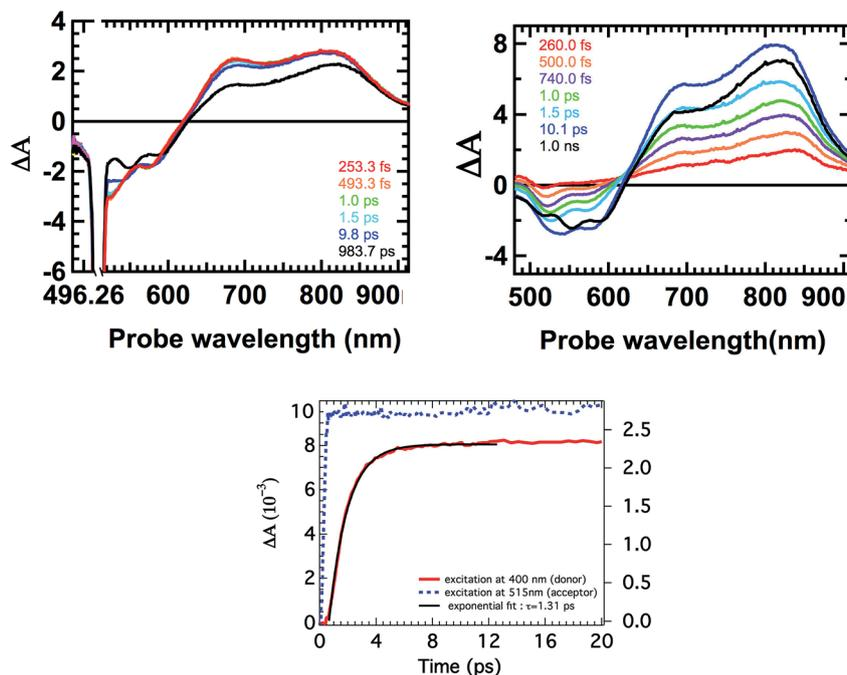
Fig. 7 Time evolution of the femtosecond transient absorption spectra of the antenna system **D1A2** after selective excitation of the perylene chromophore at 515 nm (top left) and after predominant excitation of the naphthalene chromophore at 400 nm (top right). Kinetics of **D1A2** at 820 nm obtained after excitation at 400 and 515 nm (bottom).
