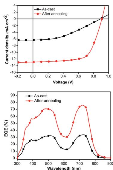
Fig. 3 The  $J$ - $V$  curves (top) and EQE plots (bottom) of the inverted devices with 4c/PC<sub>71</sub>BM (1 : 1.2, w/w) as-cast (black line) and after annealing for 5 minutes at 90 °C (red line).
