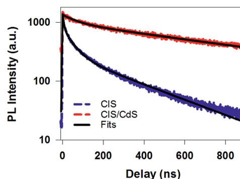
Fig. 3 Time-resolved PL decay kinetics for  $\text{CuInS}_2$  core (blue dashed line) and  $\text{CuInS}_2/\text{CdS}$  core/shell QDs (red dashed line) measured with 400 nm excitation. Their multi-exponential fits are shown in black solid lines and fitting parameters are listed in Table S1.†
