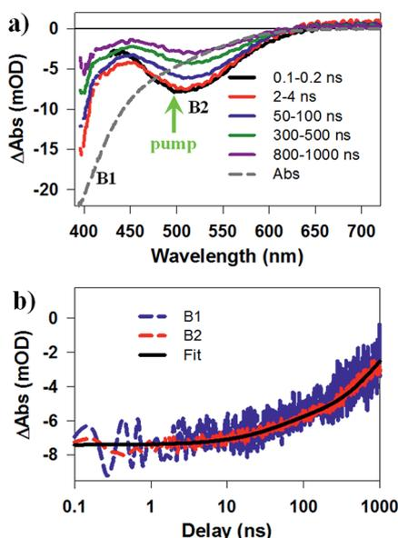
Fig. 2 Transient Absorption (TA) spectra and kinetics of  $\text{CuInS}_2/\text{CdS}$  core/shell QDs measured at 490 nm excitation. (a) TA spectra at indicated time delays (from 0.1 to 1000 ns). Static absorption spectrum (gray dashed line) is inverted and scaled for comparison. B1, B2 and excitation wavelength (green arrow) are labeled. (b) Comparison of TA kinetics of B1 (blue dashed line) and B2 (red dashed line) features and their multi-exponential fit (black solid line).
