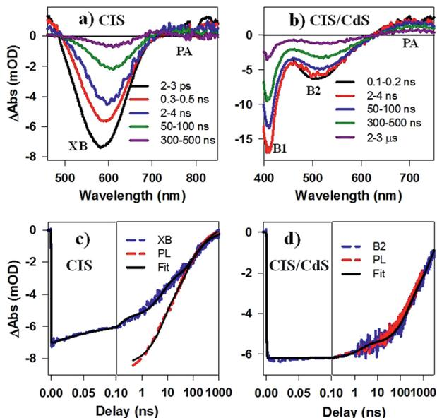
Fig. 4 TA spectra of (a)  $\text{CuInS}_2$  core, and (b)  $\text{CuInS}_2/\text{CdS}$  core/shell QDs at indicated delays after 400 nm excitation. Comparison of the kinetics of exciton bleach recovery (XB or B2, blue dashed line) and PL decay (red dashed lines) in (c)  $\text{CuInS}_2$  core, and (d)  $\text{CuInS}_2/\text{CdS}$  core/shell QDs. Their multi-exponential fits are shown in black solid lines.
