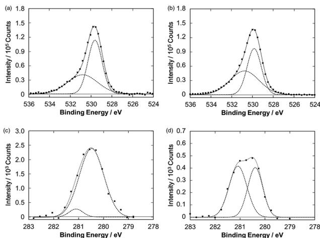
Fig. 7  $1s$  XPS spectra of the Ru–ZnP/TiO<sub>2</sub>/FTO electrodes (a) before and (b) after the PEC operation. Ru 3d<sub>5/2</sub> XPS spectra of the Ru–ZnP/TiO<sub>2</sub>/FTO electrodes (c) before and (d) after the PEC operation.
