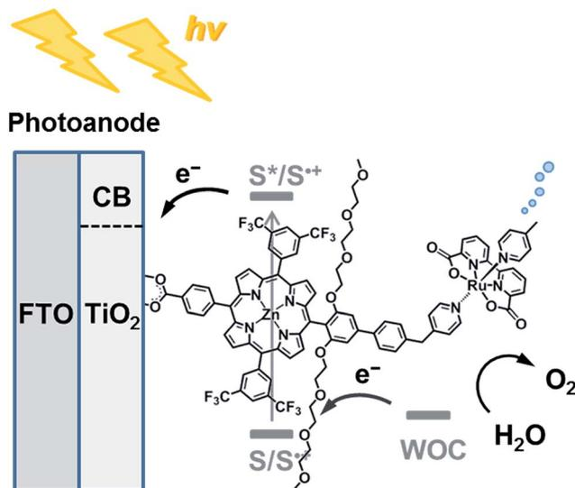
Chart 1 Schematic diagram of visible light-driven water oxidation using wide-bandgap TiO<sub>2</sub> functionalized with a ruthenium water oxidation catalyst–porphyrin linked dyad as the photoanode.
