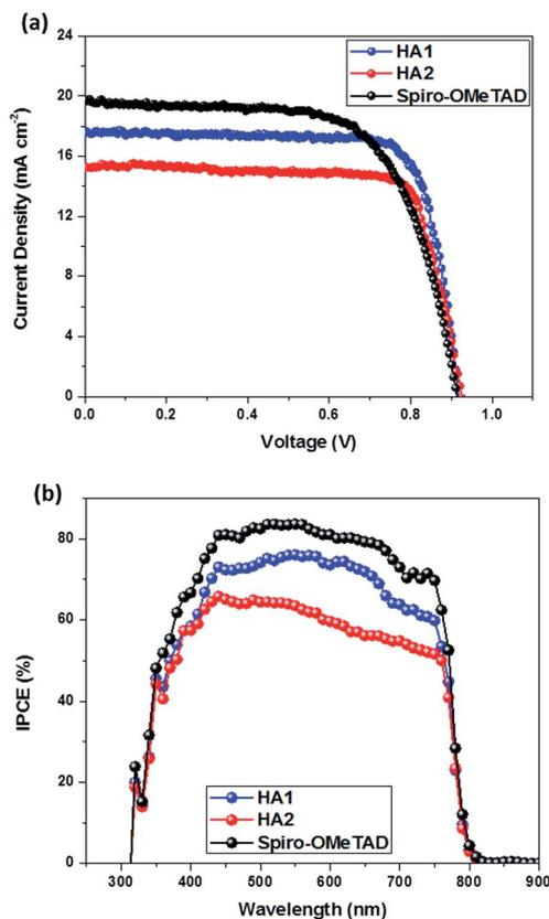
Fig. 4 (a)  $J$ - $V$  characteristics of the solar cells with HA1, HA2 and spiro-OMeTAD as the HTM. (b) The IPCE spectra of characteristics of the perovskite solar cells with HA1, HA2 and spiro-OMeTAD as the HTM.
