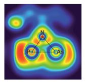
Fig. 5 ELF representation of 2P'As utilizing a phenyl substituted model compound for clarity. A section of the N-P-As plane is shown. The maximum is located aside the axis between As (left) and P (right).
