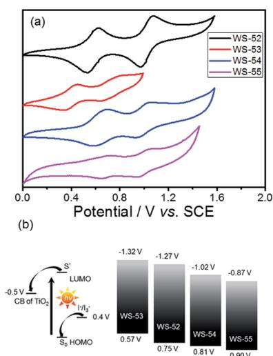
Fig. 2 (a) Cyclic voltammograms of WS-52, WS-53, WS-54 and WS-55 in  $\text{CH}_2\text{Cl}_2$ , and (b) schematic diagram of the energy levels of the  $\text{TiO}_2$  conduction band, dyes, and  $\text{I}^-/\text{I}_3^-$  redox couple.
