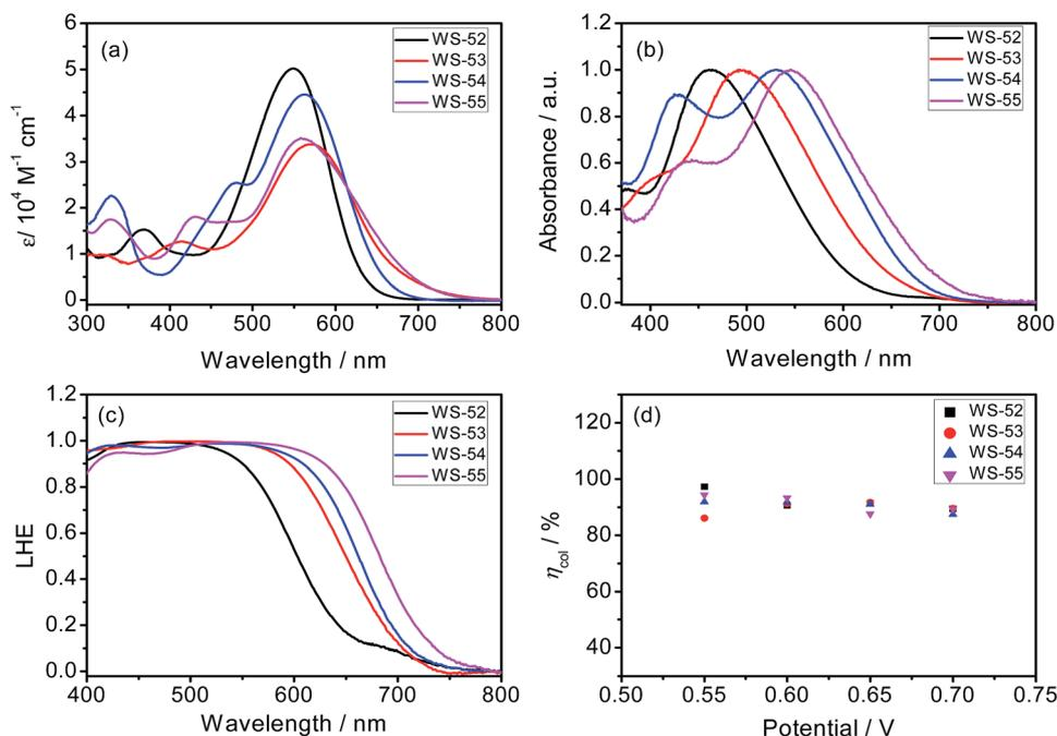
Fig. 1 Absorption spectra of **WS-52**, **WS-53**, **WS-54** and **WS-55** in  $CH_2Cl_2$  solution (a) and coated onto  $3 \mu\text{m}$   $TiO_2$  film (b), LHE spectra calculated from the absorption spectra of dye-loaded  $TiO_2$  film (c), and charge collection efficiency ( $\eta_{\text{coll}}$ ) in DSSCs as a function of bias potentials during the EIS measurement (d).
