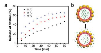
Fig. 7 (a) The release profiles of 150 kDa FD cargo from microcapsules over 1 h, at temperatures: 25, 35 and 45  $^{\circ}$ C. (b) Schematic representation of the contraction of the colloidal particles upon increasing temperature, resulting in release of encapsulated cargo.
