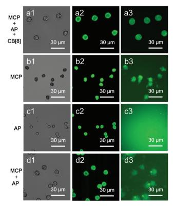
Fig. 6 (a1) Optical and (a2) fluorescence micrographs of dried supramolecular microcapsules loaded with FD (150 kDa), and (a3) after rehydration in water for 5 minutes. This is compared with microstructures prepared from microdroplets containing (b1-b3) only the MCP component, (c1-c3) only AP component, and (d1-d3) MCP and AP components in the absence of CB[8].
