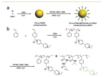
Fig. 1 (a) Schematic and (b) synthetic pathway for the preparation of the MV-bearing thermal responsive colloidal particles (MCP), *via* a styrenic templating core.
