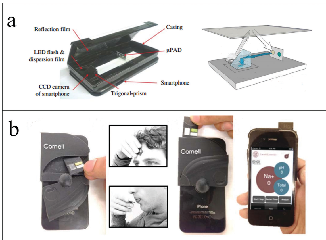
Fig. 5 MS 2 applications for routine health tests. (a) Schematic illustration of a smartphone-based optical biosensor for glucose monitoring in combination with a low-cost paper-based microfluidic device. 70 (b) Smartphone-based health sweat and saliva biomarker monitoring on the test strip. 74 The figures are adapted from ref. 70 and 74 with permission from Springer for (a) and the Royal Society of Chemistry for (b), respectively.
