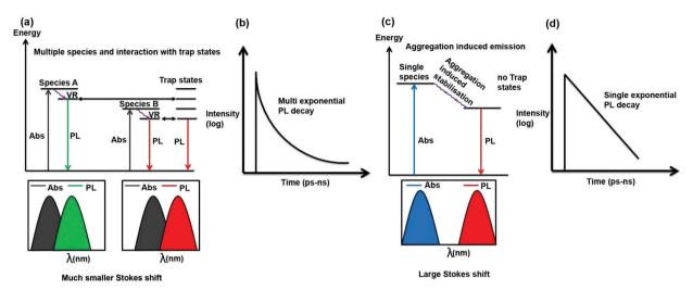
Scheme 4 Schematic showing the cause of the excitation-dependent PL emission maximum and multi-exponential PL decay (a and b). It is also shown that when the PL emission is independent of the excitation wavelength, the PL decay will be single exponential and a large Stokes shift will be observed (c and d).
