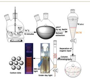
Scheme 1 Preparation and purification of orange-red emitting carbon dots using sucrose and  $\rm H_3PO_4$ .
