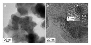
Fig. 4 TEM (a) and HRTEM (b, inset) of the VC/ac-C composite.
