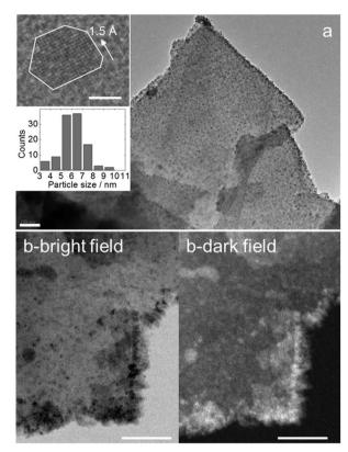
Fig. 2 (a) TEM of TiC nanoparticles on graphite (scale bar 100 nm). Top inset shows the HRTEM image of a single TiC particle with lattice fringes of  $d_{220}$ , white lines suggest the edges of the particle (scale bar 2 nm). Bottom inset shows the particle size distribution, calculated from over 100 nanoparticles. (b) STEM in a bright field (b, left) and HAADF (b, right) (scale bars: 50 nm).
