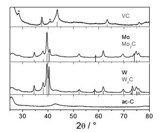
Fig. 3 PXRD patterns of ac-C/metal carbide composites with vanadium (top), molybdenum (middle) and tungsten (bottom). The reference patterns are: VC [01-089-2719] (in grey), Mo [00-001-1205] (in black),  $Mo_2C$  [04-004-8327] (in grey), W [00-004-0806] (in black), and  $W_2C$ [01-089-2371] (in grey). Stars assign reflections of KCl.
