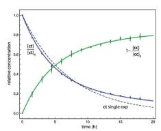
Fig. 2 Time evolution of  $H_2CO_3$  conformer concentrations in an Ar matrix at 20 K after NIR irradiation. Blue and green curves result from the global, nonlinear least-squares fit of the multi-exponential kinetic model to three and five IR bands of **1ct** and **1cc**, respectively. The dashed curve is the best single-exponential fit for **1ct**.
