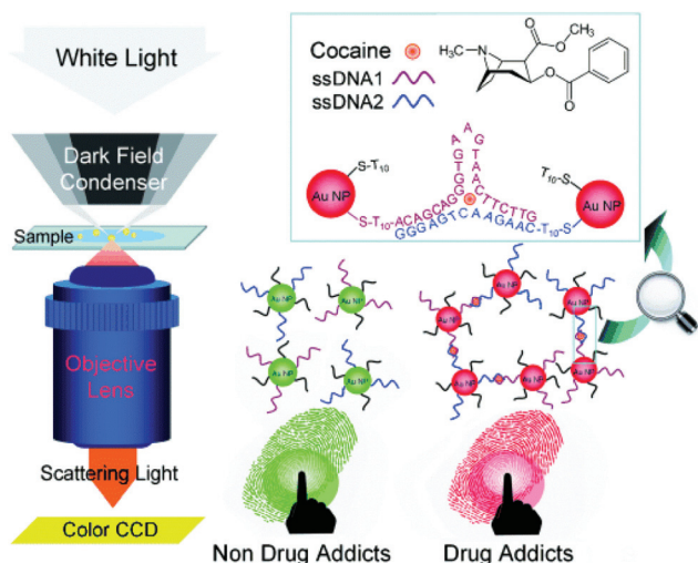
Fig. 12 Principle of the nanoplasmonic imaging of latent fingerprints and the identification of cocaine in latent fingerprints by DFM. 92 Reproduced from ref. 92 with permission from Wiley.
