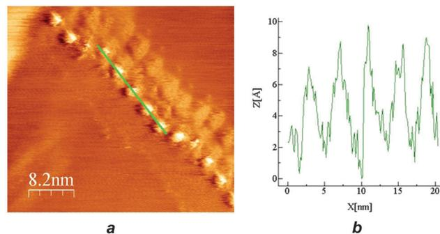
**Fig. 1** (a) STM image of a representative chain of beads from  $[\text{Fe}(\text{bpp})_2][\text{BF}_4]_2$  drop cast onto HOPG, with widths of 2.5 nm and heights of 7  $\text{Å}$ . (b) Profile over the five beads highlighted in (a).
