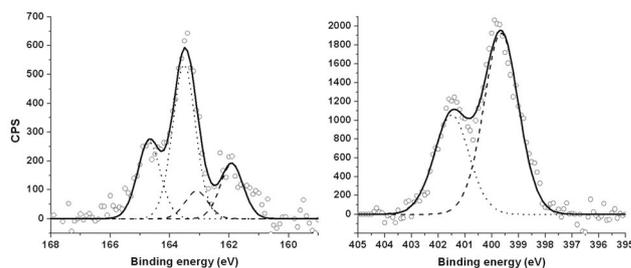
Fig. 6 High-resolution S  $2p_{3/2}$  (left) and N 1s (right) XPS data from SAMs of  $L^3$ , produced from methanol solution. Empty circles represent experimental data, dashed and dotted lines correspond to bound and unbound thiols, respectively, in S 2p region (left) and two distinct environments of nitrogen atoms in N 1s spectrum (right). Solid lines show envelopes of the fitted peaks.
