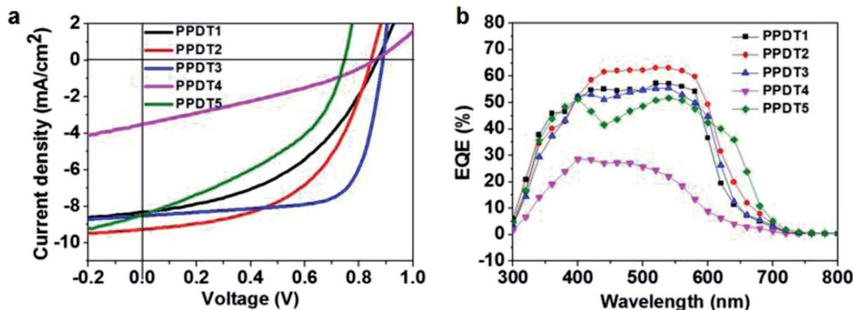
Fig. 3 (a) Current density vs. voltage characteristics of optimized PPDT : PC<sub>71</sub>BM solar cells. (b) EQE curves for the PPDT : PC<sub>71</sub>BM solar cells in (a).
