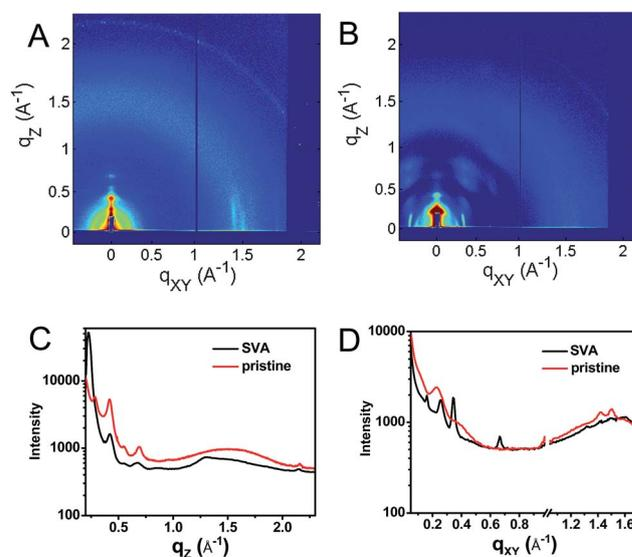
Fig. 3 GIWAXS of a pristine (A) film of **1** and a film which has been solvent vapor annealed in CH<sub>2</sub>Cl<sub>2</sub> for 10 min (B) as well as vertical (C,  $q_{xy} = 0$ ) and horizontal (D,  $q_z = 0$ ) line cuts of the annealed (black) and unannealed (red) films.
