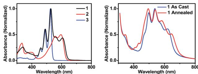
Fig. 2 UV-visible absorption spectra of molecules **1**, **2**, and **3** in toluene solution (left), and of thin films of **1** that are unannealed and  $\text{CH}_2\text{Cl}_2$  vapor annealed for 10 minutes (right).
