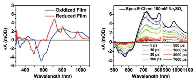
Fig. 4 (Left) A comparison of spectroelectrochemical difference spectra of **1** electrochemically oxidized and reduced in a film on ITO. (Right) A comparison of the sum of the reduced and oxidized species spectra to the fsTA spectrum of an unannealed film of **1**.
