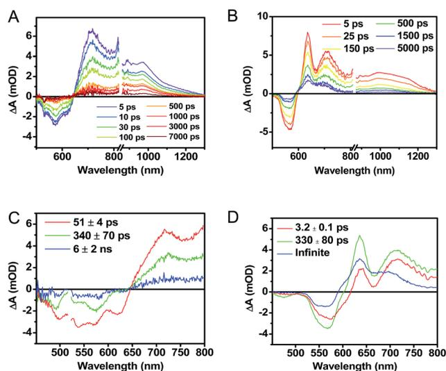
Fig. 6 fsTA spectra of an as cast, unannealed thin film of **1** (A), and a film that was solvent vapor annealed for ten minutes with  $\text{CH}_2\text{Cl}_2$  (B). Singular value decomposition (SVD) and global fitting gave decay associated spectra for the unannealed (C) and annealed (D) films.
