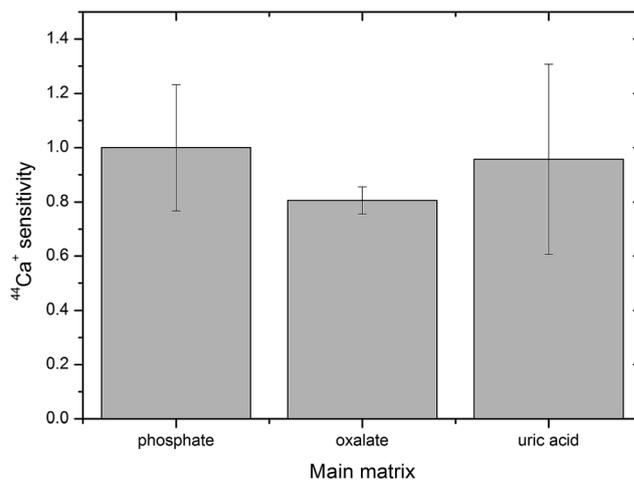
Fig. 3 Sensitivity of the calcium isotopic signal in oxalate and uric acid matrices normalized to the sensitivity in phosphate, error bars represent standard deviation.
