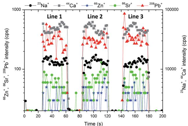
Fig. 2 The stability of the signal of <sup>23</sup>Na<sup>+</sup>, <sup>44</sup>Ca<sup>+</sup>, <sup>66</sup>Zn<sup>+</sup>, <sup>86</sup>Sr<sup>+</sup>, <sup>208</sup>Pb<sup>+</sup> during the ablation of pellet no. 7851 within 3 lines with the length of 1.5 mm, approximately.
