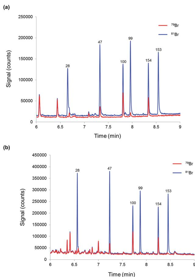
Fig. 5 Chromatograms obtained by GC-ICP-MS for (a) mineral water (blank sample) and (b) a river water sample both spiked with <sup>81</sup>Br-labelled PBDEs.
