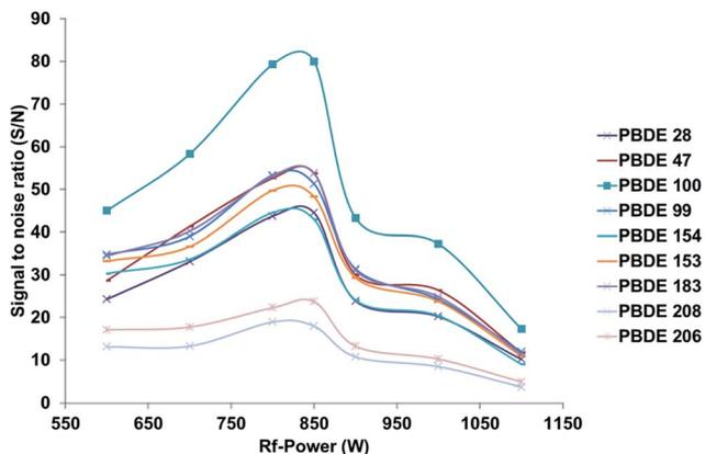
Fig. 2 Effect of the RF power settings on the signal to noise ratio of the selected PBDE congeners when using GC-ICP-MS conditions. Calculations were based on the <sup>79</sup>Br signal.
