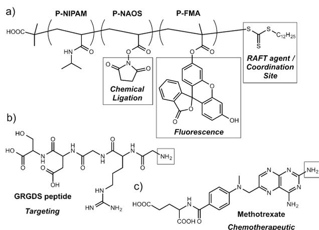
**Fig. 9** (a) Chemical structure of the RAFT random co-polymer, comprised of *N*-isopropylacrylamide (NIPAM), *N*-acryloxysuccinimide (NAOS), and fluorescein-*O*-methacrylate (FMA) monomers, used to coat [Gd(1,4-bdc)<sub>1.5</sub>(H<sub>2</sub>O)<sub>2</sub>]<sub>n</sub> nanoparticles. The activated NHS ester allows post-synthetic conjugation of (b) targeting GRGDS peptides and (c) methotrexate chemotherapeutic units through reaction with free amino groups.
