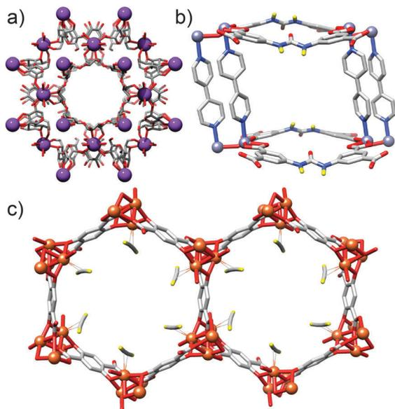
**Fig. 1** Sections of the solid-state structures of (a) CD-MOF-2, whose surfeit of pendant hydroxyl units facilitates transient chemisorption of CO<sub>2</sub>, (b) NU-601, a urea functionalised MOF which acts as a heterogeneous organocatalyst, and (c) iron dioxidoterephthalate, binding acetylene through interactions with coordinatively unsaturated Fe<sup>2+</sup> cations. Redrawn from CSD depositions LAJLEP, HAPHUD and SARGID, in turn.
