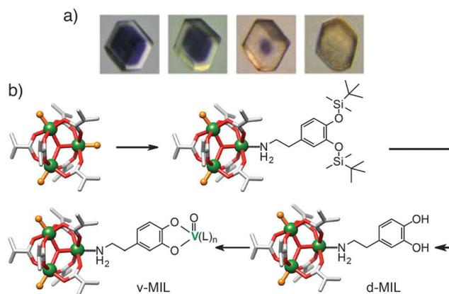
**Fig. 13** (a) Photographs of metal cation exchange in  $[\text{Co}_6(1,3,5\text{-btb})_4(4,4'\text{-bipy})_3]_n$ , occurring from the surface of the crystal inwards. Reprinted (adapted) with permission from ref. 51. Copyright (2012) American Chemical Society. (b) Scheme showing coordination of bulky TBDMS-protected dopamine to the  $\text{Cr}^{3+}$  cations of the SBUs at the surface of MIL-101(Cr) only, which can then be deprotected and vanadylated.
