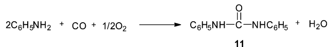
Scheme 5 Reagents and conditions: aniline (53.8 mmol), catalyst 5% Pd/C ( 5.0 \times 10^{-3} \text{ g cm}^{-3} ), NaI (0.87 mmol), DMF ( 95 \text{ cm}^3 ), \text{CO} : \text{O}_2 pressure (41 bar) ( \text{CO} : \text{O}_2 , 5 : 1), temp. 100^\circ\text{C} , time 2 h.
