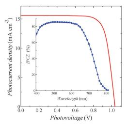
Fig. 3 Typical I-V properties of the ADEKA-1-sensitized solar cell with the highest efficiency of 12.5% (entry 8 in Table 1) under the simulated one sun irradiation (AM-1.5G, 100 mW cm<sup>-2</sup>). Inset shows the IPCE spectrum of the cell.
