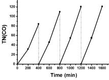
Fig. 3 Formation of CO in a 4-cycle repetition of irradiation at >420 nm for 400 min after CO<sub>2</sub> bubbling for 30 min in the dark; 10 mg Dye/S-TiO<sub>2</sub>/ ReC with 0.1  $\mu\text{mol}$  ReC and 1.5  $\mu\text{mol}$  Dye in the presence of 0.1 M SD and 10% (v/v) H<sub>2</sub>O
