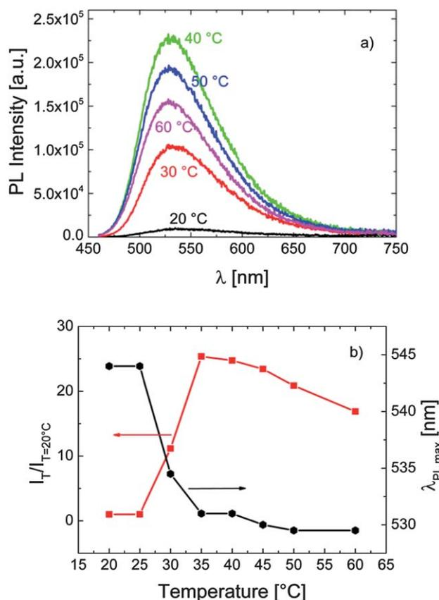
**Fig. 2** (a) The evolution of the fluorescence spectrum of **P-1** in PBS (0.1 g L<sup>-1</sup>) with temperature, recorded at an excitation wavelength of 450 nm. (b) The correlation between  $\lambda_{\text{PL,max}}^{\text{PL}}$ , the relative emission intensity ( $I_T/I_{T=20\text{ °C}}$ ), and the temperature of the solution. Data are taken from the spectra in (a).
