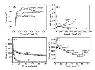
**Fig. 4** (a) Cyclic voltammetry profiles of the Si/TRG composites and (b) galvanostatic discharge–charge curves for different cycles. (c) Cycling performance of the Si/TRG composites and Si nanoparticles. (d) Rate capability of the Si/TRG composites.
