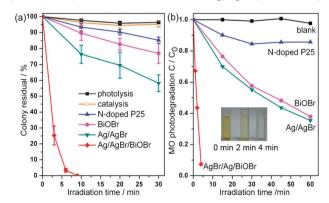
Fig. 3 Photocatalytic (a) inactivation of E. coli and (b) degradation of MO under visible light irradiation ( $\lambda \geq 400$  nm). The insert demonstrates the color changes of MO over Ag/AgBr/BiOBr hybrid.
