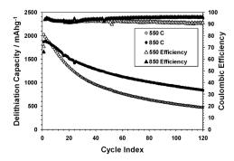
**Fig. 4** Delithiation capacities and coulomb efficiencies of SG samples reduced at 550 or 850 °C, using a constant current–constant voltage (CCCV) method (1.5–0.020 V, 1000–50 mA g $^{-1}$ ).
