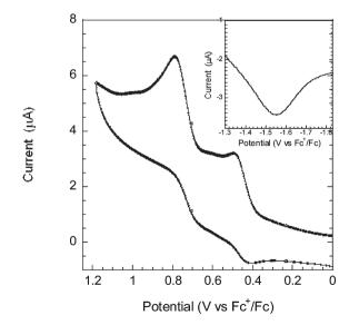
Fig. 3 Cyclic voltammogram of the oxidation behaviour and square wave voltammogram (inset) of the reduction, measured at a scan rate of  $100 \text{ mV s}^{-1}$ . The formal potentials of oxidation and reduction were determined to 450 mV and -1550 mV vs. Fc<sup>+</sup>/Fc.
