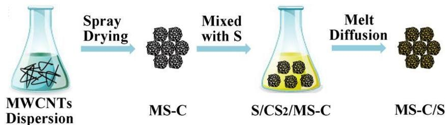
**Scheme 1.** Schematic illustration of the synthesis process of the MS-C/S
