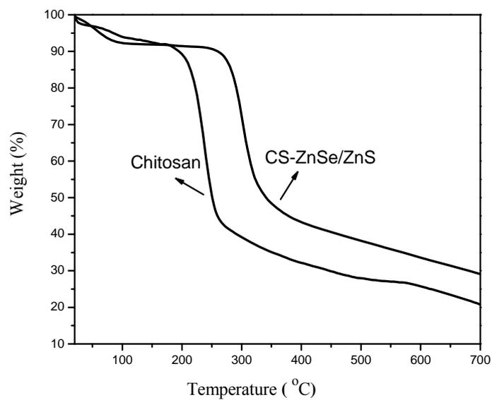
Fig. 6 TG curves of pure chitosan and CS-ZnSe/ZnS nanoparticles.
