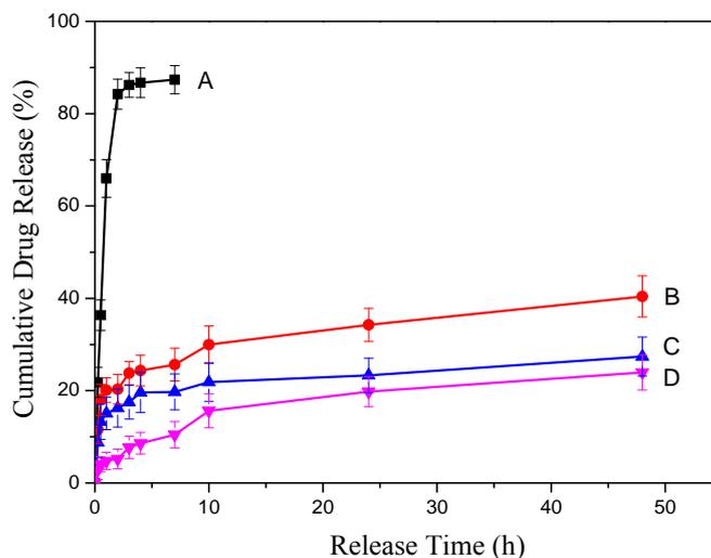
Fig. 8 Cumulative release curve of samples in pH 7.4 (PBS) at 37 °C: (A) bare 5-Fu, (B) 5-Fu-CS-ZnSe/ZnS nanoparticles obtained from 4 mg·mL<sup>-1</sup> ZnSe/ZnS QDs, (C) 5-Fu-CS-ZnSe/ZnS nanoparticles obtained from 8 mg·mL<sup>-1</sup> ZnSe/ZnS QDs, (D) 5-Fu-CS-ZnSe/ZnS nanoparticles obtained from 12 mg·mL<sup>-1</sup> ZnSe/ZnS QDs.
