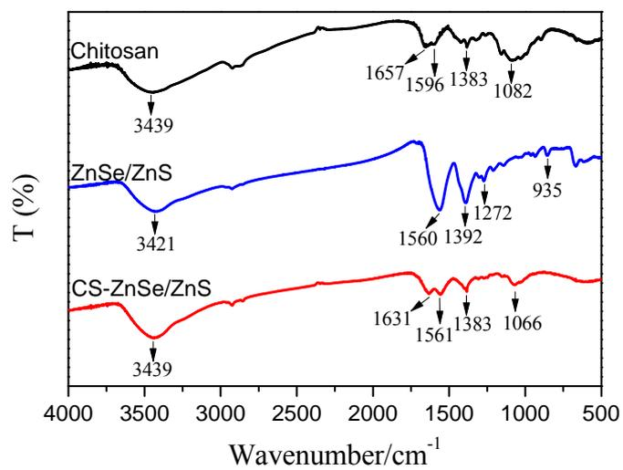
Fig. 4 FT-IR spectra of pure chitosan, ZnSe/ZnS QDs and CS-ZnSe/ZnS nanoparticles.
