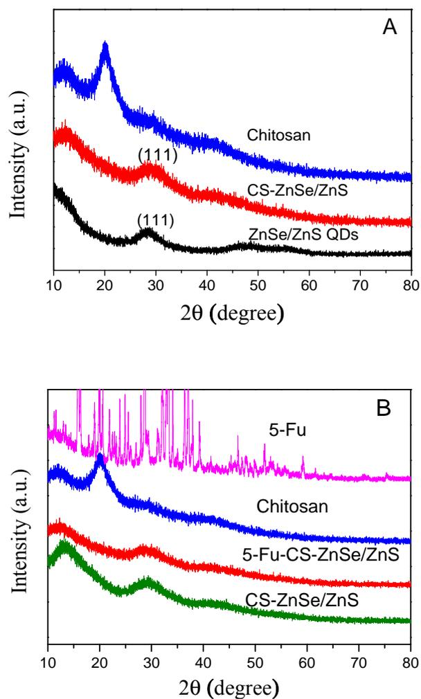
Fig. 2(A) XRD patterns of chitosan, ZnSe/ZnS QDs, CS-ZnSe/ZnS nanoparticles and (B) XRD patterns of pure 5-Fu, chitosan, fluorescent CS-ZnSe/ZnS nanoparticles and 5-Fu-CS-ZnSe/ZnS nanoparticles.
