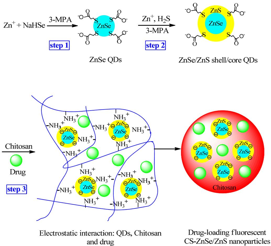
Fig. 1 Schematic representation of the fabrication process of drug-loading fluorescent CS-ZnSe/ZnS nanoparticles.
