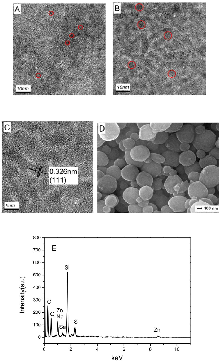
Fig. 3(A) TEM images of ZnSe QDs (B, C) TEM and HRTEM images of ZnSe/ZnS QDs, (D) SEM image of CS-ZnSe/ZnS nanoparticles and (E) EDX spectrum of CS-ZnSe/ZnS nanoparticles.
