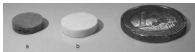
Fig. 4 Pellet of poly(aminoborane) 7 (R = H) (a) after pyrolysis at 900 °C, (b) before pyrolysis. The Euro coin is shown for scale. Reproduced from Ref. 40 with permission of John Wiley and Sons.
