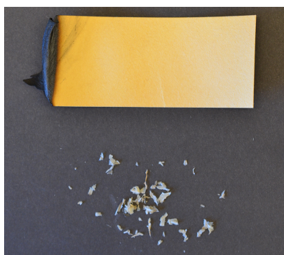
Fig. 12 Top: Dynamic sheet formed (DSF) paper made from thermomechanical pulp (TMP) was coated with poly(methylenephosphine oxide) 70a (0.8 mmol P / g) and ignited with a lighter in air. This flame retardant paper is self-extinguishing. Bottom: An untreated DSF TMP sheet was ignited in air and burns completely.
