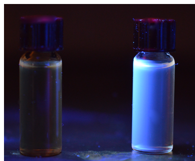
Fig. 13 A photograph showing (left) a THF solution of poly( p -phenylenediethynylene phosphine) 76 ( R = \text{C}_6\text{H}_{13} ) and (right) an analogous solution of the phosphine oxide 76-O . Both samples are being irradiated with a UV lamp.
