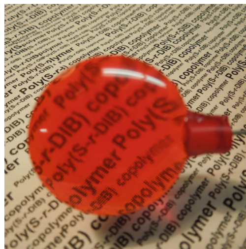
Fig. 16 Film of inverse vulcanized polysulfur 94 . Image provided courtesy of Prof. J. Pyun.
