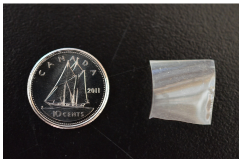
Fig. 11 Film cast from a block copolymer of phosphalkene and styrene. Photograph provided courtesy of Dr. E. Conrad.
