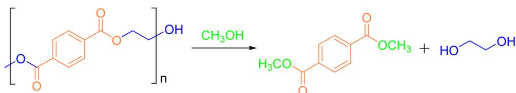
Fig. 3 The reaction formula of methanol alcoholysis.
