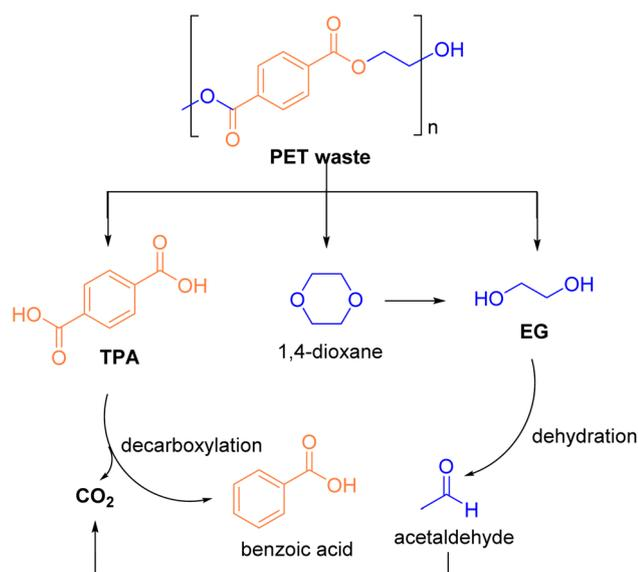
Fig. 13 Potential pathways for PET waste under sub- and supercritical water. Reproduced with permission.<sup>100</sup> Copyright 2020, Elsevier Ltd.
