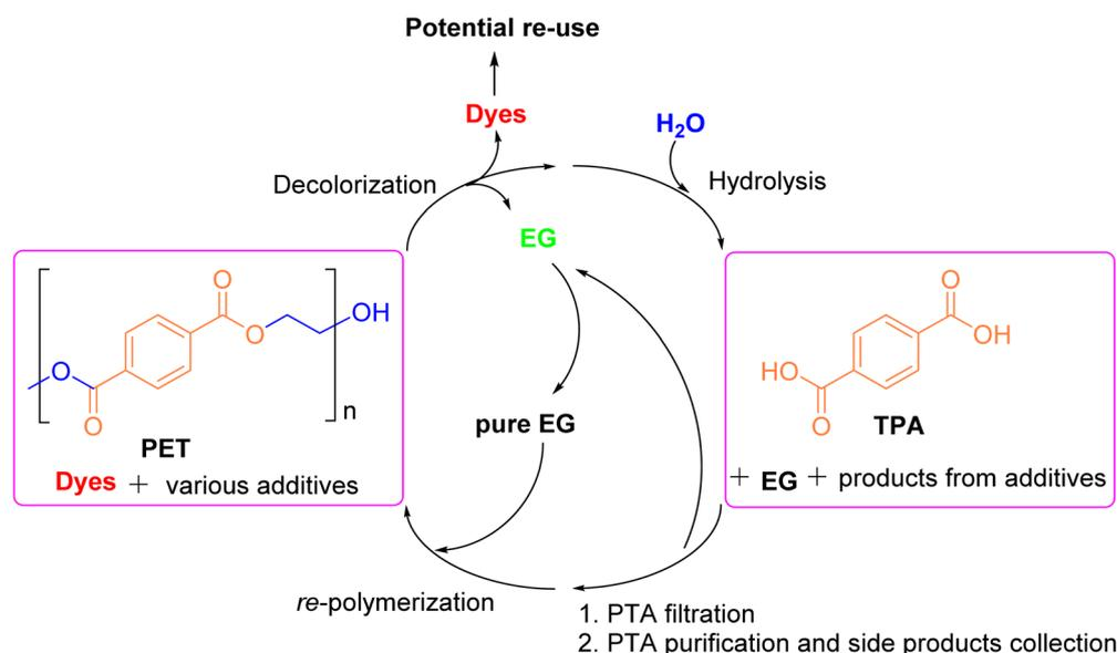
Fig. 12 A closed-loop route for recycling waste polyester textiles that includes pre-decolorization, neutral hydrolysis, PTA purification, and chemicals recovery. Reproduced with permission.<sup>104</sup> Copyright 2024, Elsevier Ltd.
