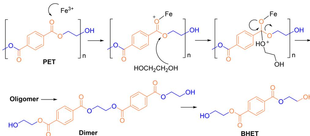
Fig. 8 Glycolysis mechanism of PET using Fe<sub>2</sub>O<sub>3</sub> nanoparticles as catalysts. Reproduced with permission.<sup>63</sup> Copyright 2021, the Royal Society of Chemistry.
