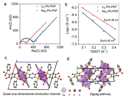
Fig. 3 (a) Nyquist plots for Li<sub>4</sub>-Ph-PhP and Na<sub>4</sub>-Ph-PhP at 30 °C, (b) Arrhenius plot of ionic conductivity of A<sub>4</sub>-Ph-PhP (A = Li, Na), (c and d) structural representation of Na<sub>4</sub>-Ph-PhP highlighting the one-dimensional Na chain along the b axis.
