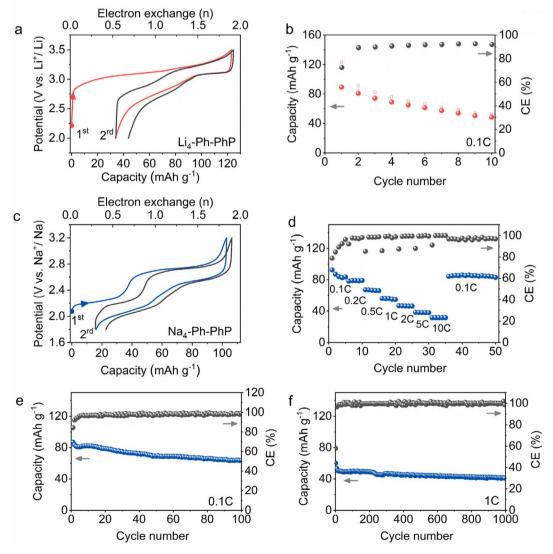
Fig. 4 Electrochemical performance of  $Li_4$ -Ph-PhP and  $Na_4$ -Ph-PhP as positive electrode materials for charge storage.  $Li_4$ -Ph-PhP: (a) the first two charge and discharge voltage profiles at 0.1C and (b) cycling performance at 0.1C;  $Na_4$ -Ph-PhP: (c) the first two charge and discharge voltage profiles at 0.1C, (d) capacity-rate from 0.1C to 10C per series of five cycles, and cycling performance at (e) 0.1C and (f) 1C.
