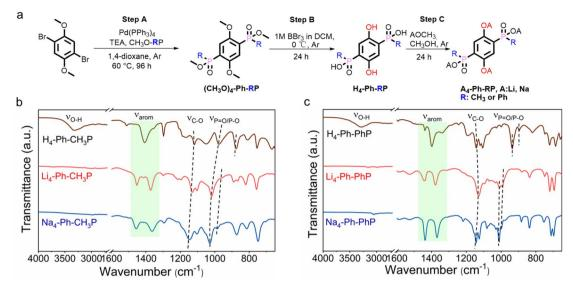
Fig. 1 (a) Synthetic pathway for  $A_4$ -Ph-RP, A = Li or Na and  $R = CH_3$  or Ph. Comparative FTIR analysis of the methyl version (b) and the phenyl version (c) and their corresponding lithium and sodium salts.
