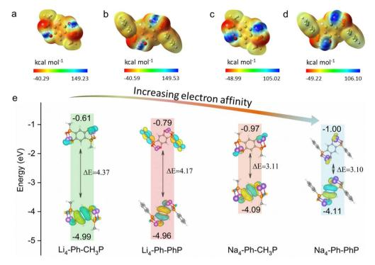
Calculated ESP maps of (a) Li<sub>4</sub>-Ph-CH<sub>3</sub>P, (b) Li<sub>4</sub>-Ph-PhP, (c) Na<sub>4</sub>-Ph-CH<sub>3</sub>P and (d) Na<sub>4</sub>-Ph-PhP, (e) HOMO-LUMO energy level diagram.
