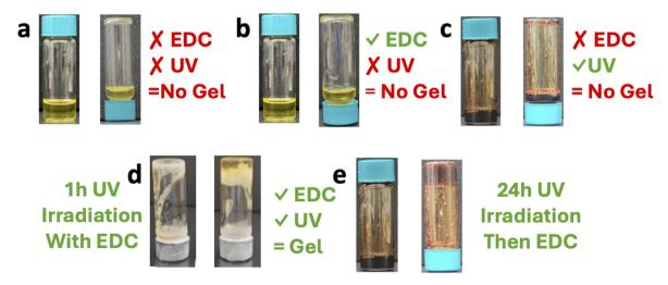
Fig. 1 Inverted vial tests for (a) protected poly(ONBM<sub>15</sub>-DMAm<sub>81</sub>) without the addition of EDC, (b) protected poly(ONBM<sub>15</sub>-DMAm<sub>85</sub>) with EDC added, (c) deprotected poly(ONBM<sub>15</sub>-DMAm<sub>81</sub>) without EDC, (d) protected poly(ONBM<sub>15</sub>-DMAm<sub>81</sub>) with EDC added then exposed to 360 nm UV for 1 h, and (e) deprotected poly(ONBM<sub>15</sub>-DMAm<sub>81</sub>) with EDC added.
