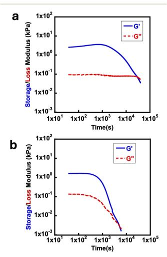
Fig. 4 Typical rheology time sweeps at 15 °C using a frequency of 10 rad  $s^{-1}$  with 1 M EDC for deprotected (a) poly(ONBM<sub>15</sub>-DMAm<sub>81</sub>) and (b) poly(ONBM<sub>15</sub>-DMAm<sub>122</sub>).
