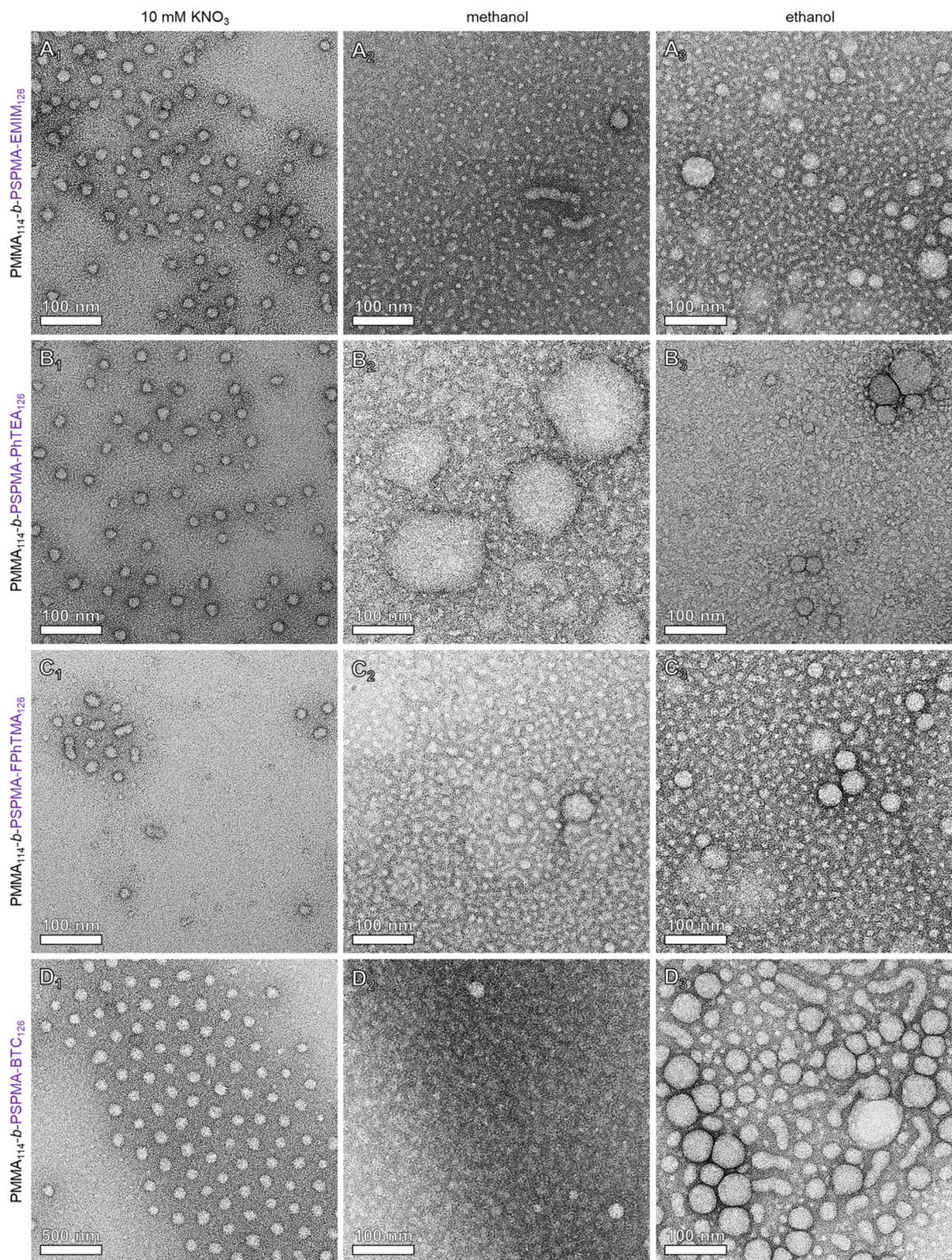
**Fig. 5** Comparative self-assembly of amphiphilic block copolymers in various types of media. Negatively stained TEM images of polymer micelles obtained from (A) PMMA<sub>114</sub>-*b*-PSPMA-EMIM<sub>126</sub>, (B) PMMA<sub>114</sub>-*b*-PSPMA-PhTEA<sub>126</sub>, (C) PMMA<sub>114</sub>-*b*-PSPMA-FPhTMA<sub>126</sub> and (D) PMMA<sub>114</sub>-*b*-PSPMA-BTC<sub>126</sub> in 10 mM KNO<sub>3</sub>, methanol or ethanol.
