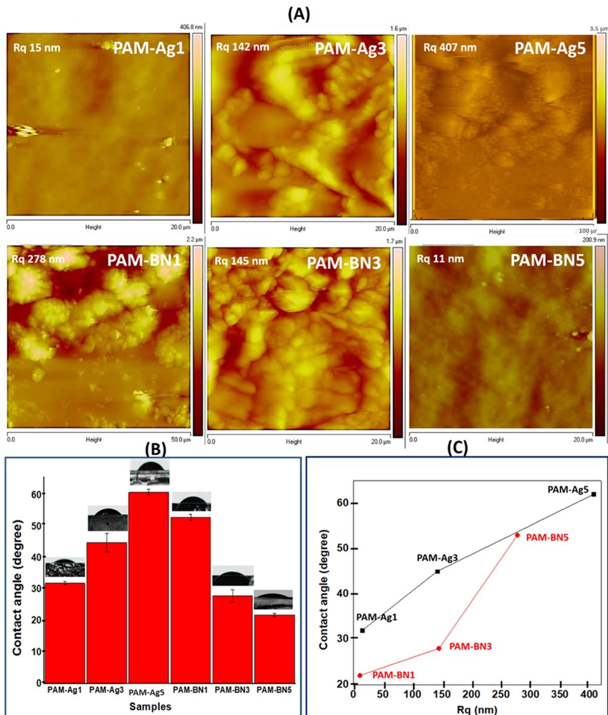
**Fig. 5** (A) AFM topographies of the engineered hydrogel surfaces, (B) contact angle values and (C) connections between surface roughness and water contact angles measured through all designed Ag and BN-based hydrogel samples.
