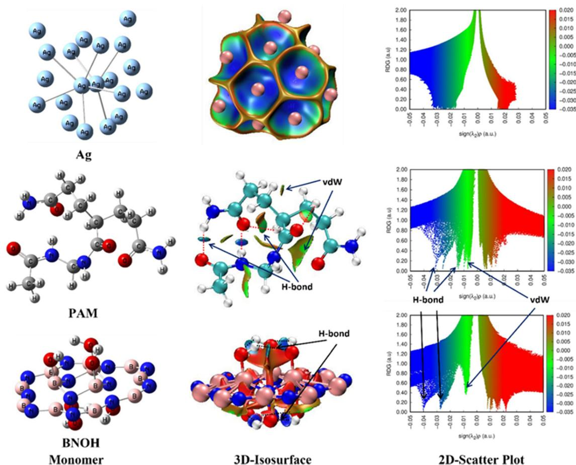
**Fig. 14** Optimized/equilibrium structures of the Ag (top-left), PAM (middle-left) and BNOH (below-left) models at the B3LYP/6-31G level of theory along with their respective NCI-plots, 3D-isosurface maps (middle) and 2D-scatter plots (right).
