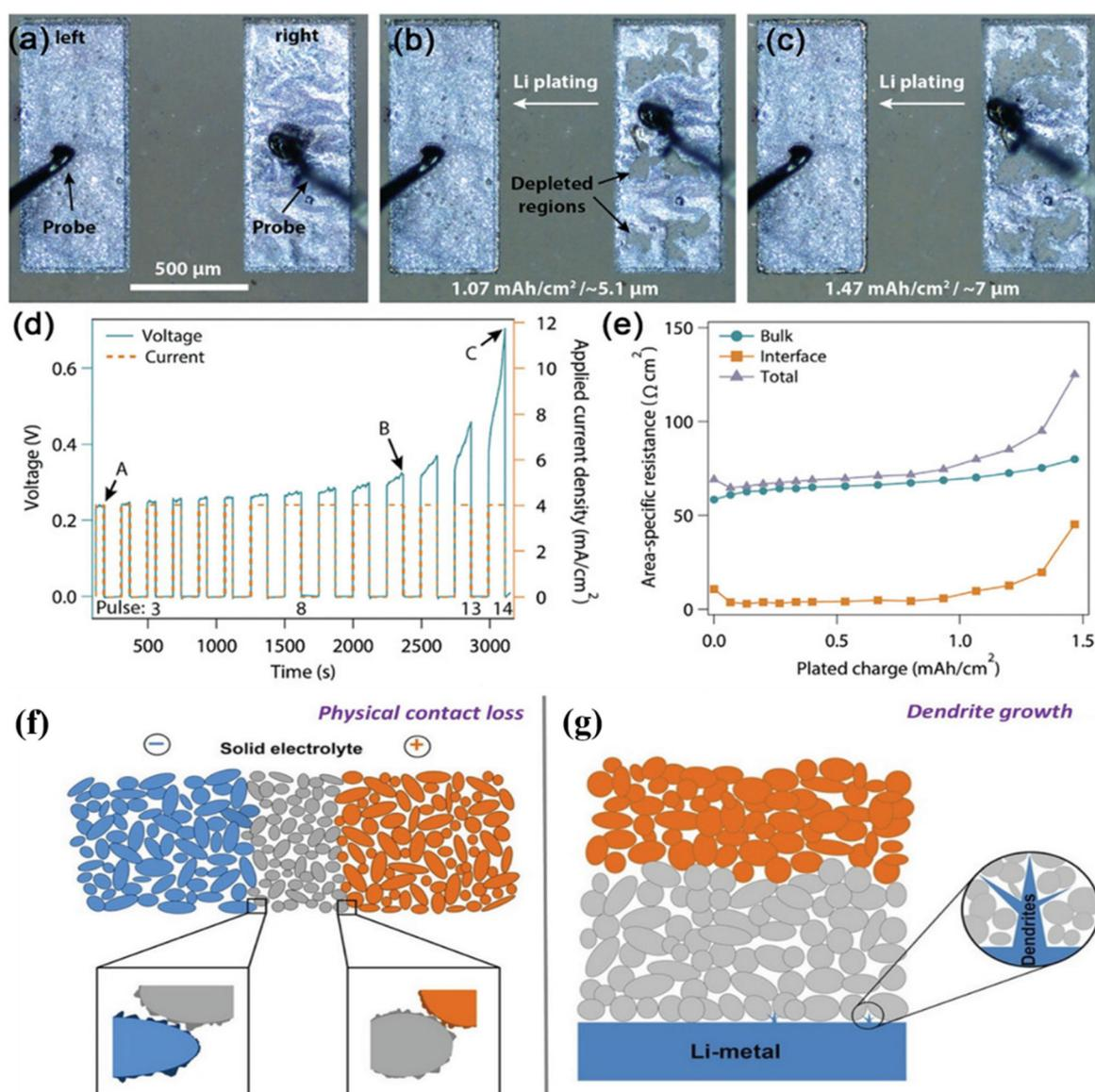
**Fig. 6** Contact loss at the anode in ASSLBs. (a) Microelectrode arrangement for experimental use. Depletion regions of (b) 1.07 mA h cm<sup>-2</sup> stripping and (c) 1.47 mA h cm<sup>-2</sup>. (d) Increase in polarization following contact losses. (e) Rise of impedance with continuous stripping.<sup>138</sup> Schematic illustrations demonstrate physical contact losses in ASSLBs (f) and dendrite evolution within ASSLBs (g).<sup>141</sup>
