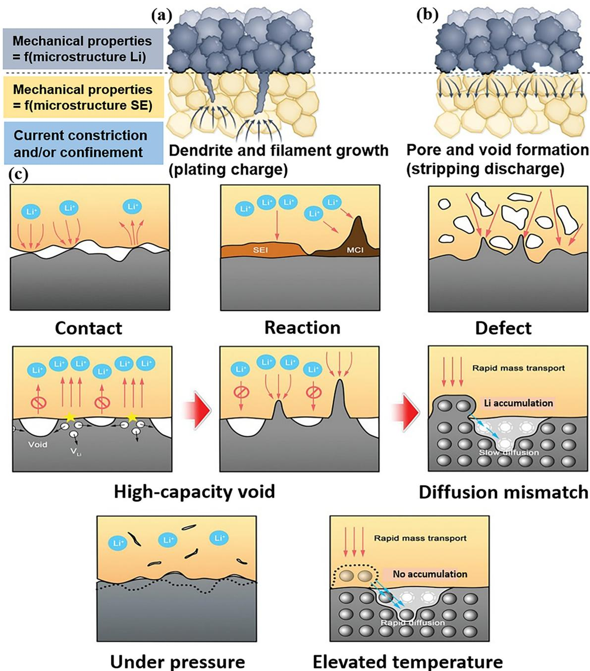
**Fig. 5** Crucial concerns with the lithium metal anode. (a) Filament and dendrite development. (b) Pore and void development.<sup>140</sup> (c) Scheme illustrating the main factors affecting CCD.<sup>50</sup>
