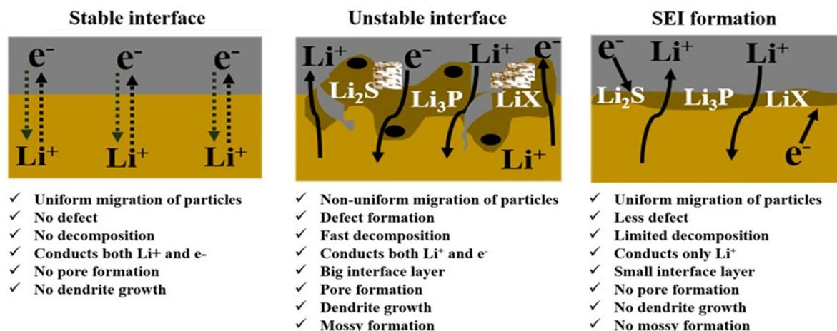
Fig. 2 Scheme illustrating the three possible types of interface between  $\text{Li}_6\text{PS}_5\text{X}$  (X = Cl, Br, I) and lithium.
