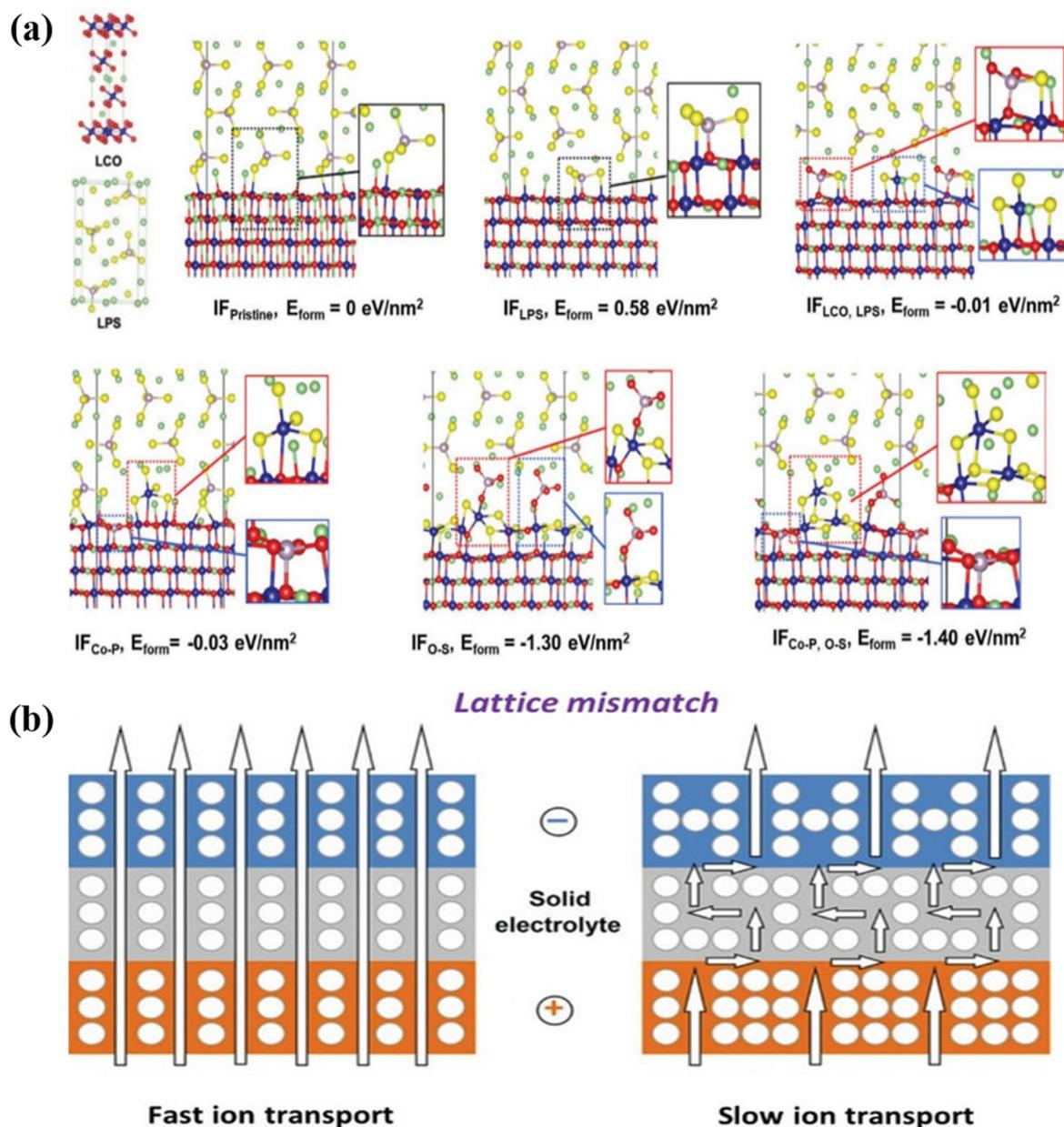
Fig. 8 (a) Predicted low-energy interface structures between  $\text{LiCoO}_2$  and  $\text{Li}_3\text{PS}_4$  for six different energy states.<sup>177</sup> (b) Lattice (mis)match.<sup>141</sup>
