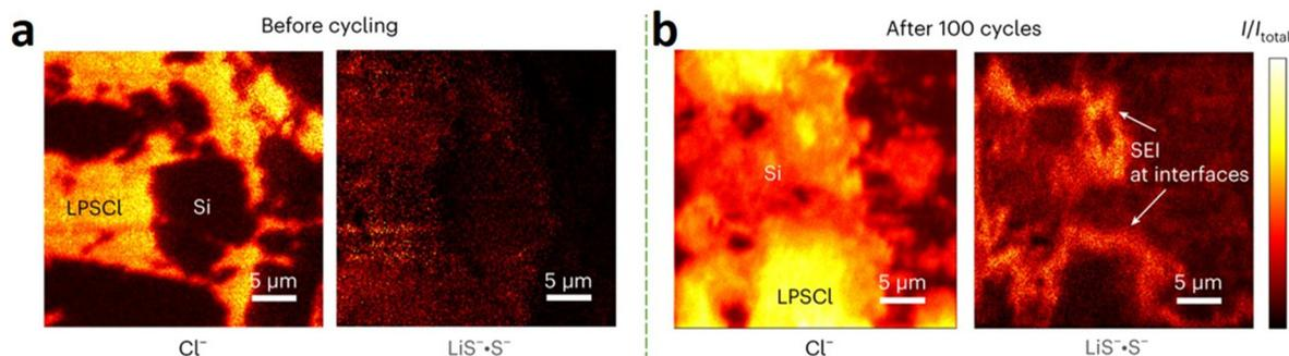
Fig. 32 ToF-SIMS images of the  $\text{Cl}^-$  fracture and the product of the  $\text{LiS}^+$  and  $\text{S}^-$  fractures in Si/Li<sub>6</sub>PS<sub>5</sub>Cl composites before cycling (a) and after 100 cycles (b).<sup>362</sup>
