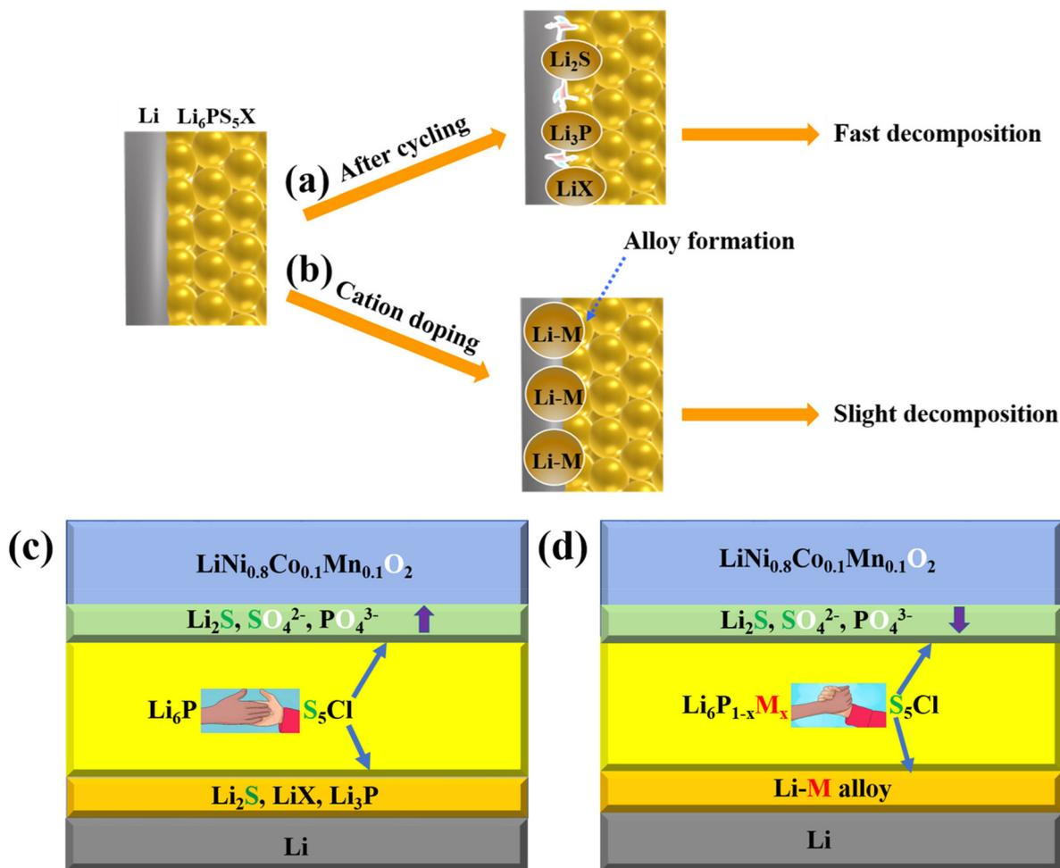
**Fig. 16** Scheme illustrating the role of cation-substituted  $\text{Li}_6\text{PS}_5\text{X}$  (X = Cl, Br, I) SEs. Anode side interface: (a) bare and (b) cation-doped SEs towards Li metal after cycling. Cathode side interface: (c) bare and (d) cation-doped electrolyte with layered oxide cathode materials after cycling.
