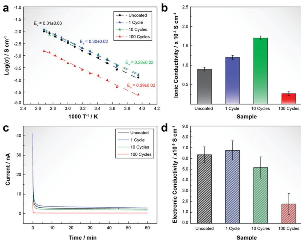
**Fig. 11** (a) Arrhenius plots, (b) ionic conductivity at 25 °C, (c) current–time curves (DC polarization at 200 mV, 25 °C) and (d) electronic conductivity at 25 °C for  $\text{Li}_6\text{PS}_5\text{Cl}$  pellets pressed from powders coated with 1, 10, and 100 ALD alumina cycles in comparison with pellets pressed from uncoated powders.<sup>226</sup>
