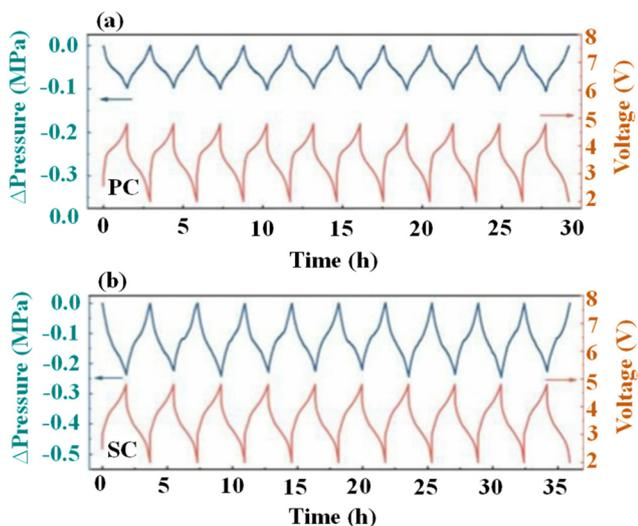
Fig. 26 Operando pressure curves of (a) PC- and (b) SC-Li<sub>1.2</sub>Ni<sub>0.13</sub>Mn<sub>0.54</sub>Co<sub>0.13</sub>O<sub>2</sub> in Li<sub>4</sub>Ti<sub>5</sub>O<sub>12</sub>|Li<sub>6</sub>PS<sub>5</sub>Cl|Li<sub>1.2</sub>Ni<sub>0.13</sub>Mn<sub>0.54</sub>Co<sub>0.13</sub>O<sub>2</sub> cells.<sup>335</sup>
