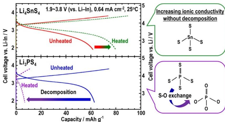
Fig. 18 The role of cation dopant in thermal stability.<sup>305</sup>
