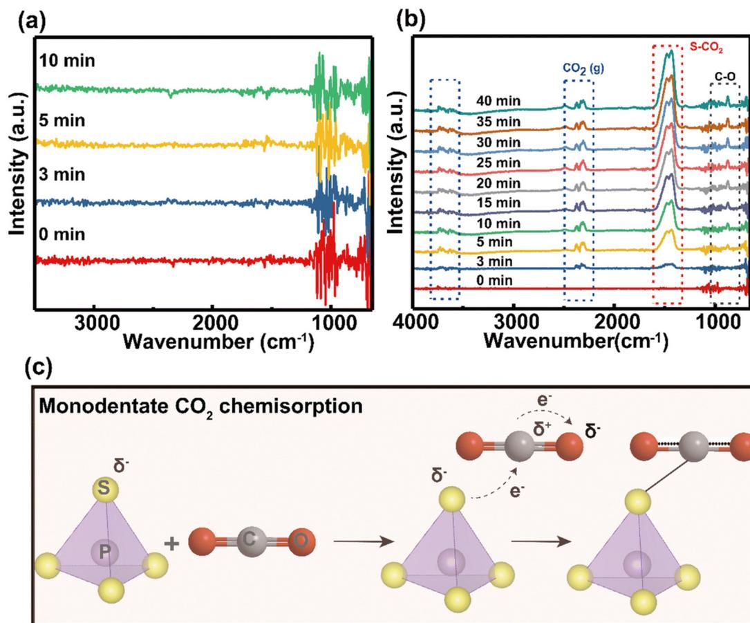
Fig. 25 *In situ* DRIFTS measurements. The *in situ* DRIFTS findings of CO<sub>2</sub> adsorption on Li<sub>6</sub>PS<sub>5</sub>Cl at 150 °C show: (a) the initial conditions under Ar purging and (b) the spectral alterations for Li<sub>6</sub>PS<sub>5</sub>Cl when CO<sub>2</sub> is purged at a rate of 30 c.c. min<sup>-1</sup>. (c) A depiction of monodentate CO<sub>2</sub> chemisorption on Li<sub>6</sub>PS<sub>5</sub>Cl is also provided.<sup>334</sup>
