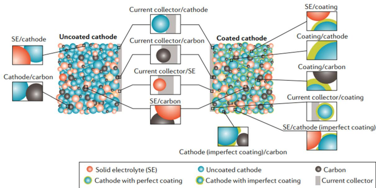
Fig. 14 Interfaces within cathode composites. A schematic representation of the different cathode composite interfaces within ASSLBs, both with and without cathode coatings.<sup>63</sup>
