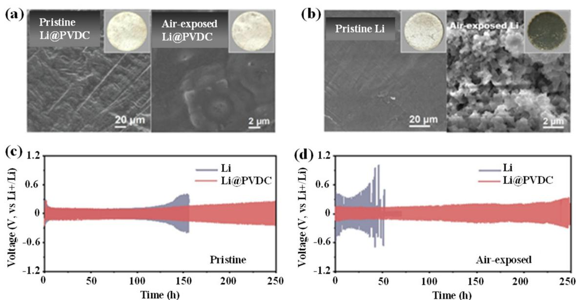
**Fig. 13** The role of interlayers in suppressing air corrosion in the lithium metal anode. SEM images of (a) Li@PVDC and (b) bare lithium before and after exposure to ambient air for 30 min. Voltage profiles of bare lithium and Li@PVDC symmetric cells (c) without and (d) with 30 min air exposure at  $1 \text{ mA cm}^{-2}$  and  $1 \text{ mAh cm}^{-2}$ .<sup>262</sup>
