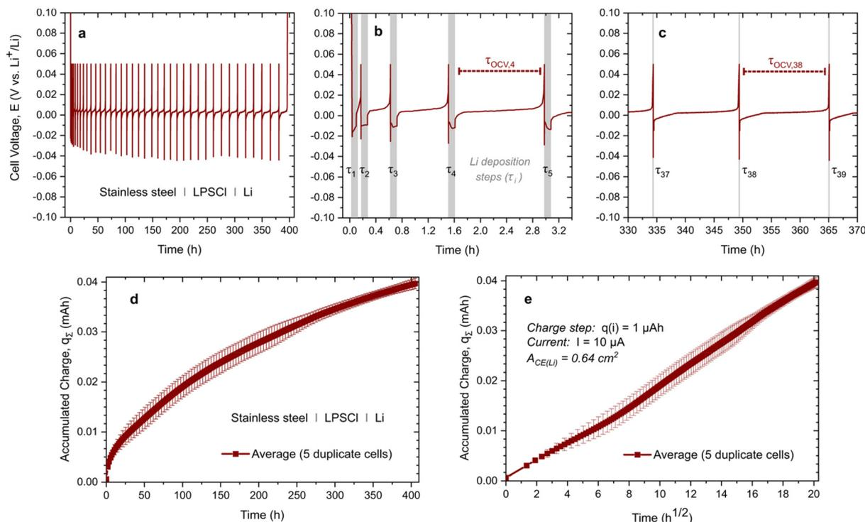
**Fig. 20** CTTA measurements. (a) Output for the LPSCI SE in a stainless steel/LPSCI/Li assembly at a temperature of 25 °C and pressure of approximately 13 MPa. The potential profiles are depicted for two distinct time intervals: an early stage (b) and a later stage (c) of the measurement. The total stored capacity over time is illustrated in (d) as a function of time and (e) as a function of the square root of time.<sup>316</sup>
