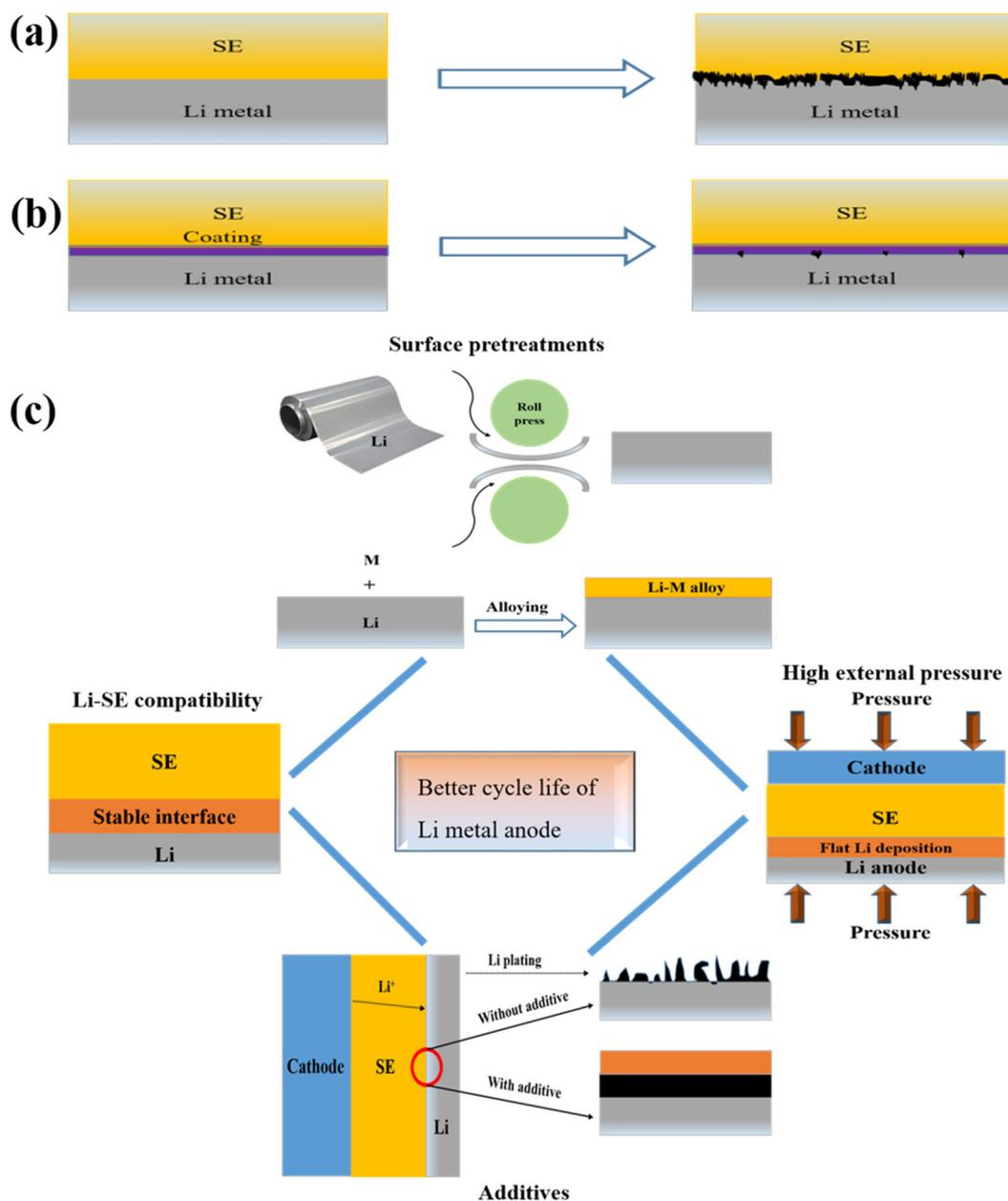
**Fig. 12** (a) Porous surface of the electroplated lithium anode after extended cycling. (b) The dense surface of the lithium anode is electroplated underneath the protective coating. (c) Approaches for enhancing the cycling span of lithium metal anodes.
