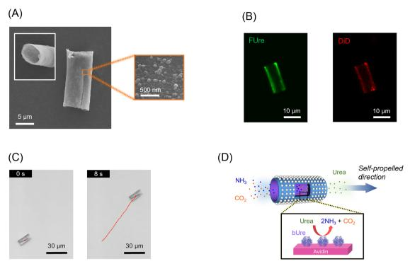
Fig. 6 (A) SEM images of DoxL/Ure tubes. (B) CLSM images of DoxL/FUre tubes. Green fluorescence: FUre; red fluorescence: DiD. (C) Microscopic observation of a DoxL/Ure tube micromotor with trajectory in PBS solution ([urea] = 100 mM). (D) Schematic illustration of DoxL/Ure tube micromotor propulsion via urea decomposition into NH<sub>3</sub> and CO<sub>2</sub>. From ref. 106. Copyright 2025, American Chemical Society,
