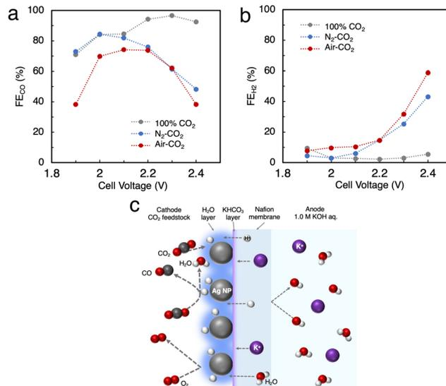
Fig. 5 (a) FE for CO production (FE<sub>CO</sub>) and (b) for the HER (FE<sub>H<sub>2</sub></sub>) in the CO<sub>2</sub>RR using N<sub>2</sub>-CO<sub>2</sub> and air-CO<sub>2</sub>. (c) Predicted mechanism of the CO<sub>2</sub>RR on the Ag MEA-cell.
