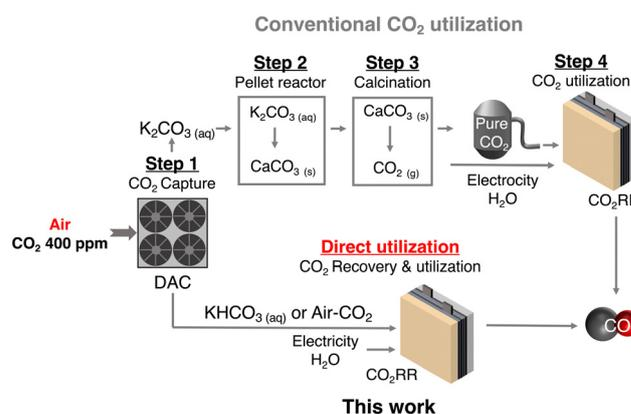
Fig. 1 Scheme of recovery and utilization of atmospheric CO<sub>2</sub>.
