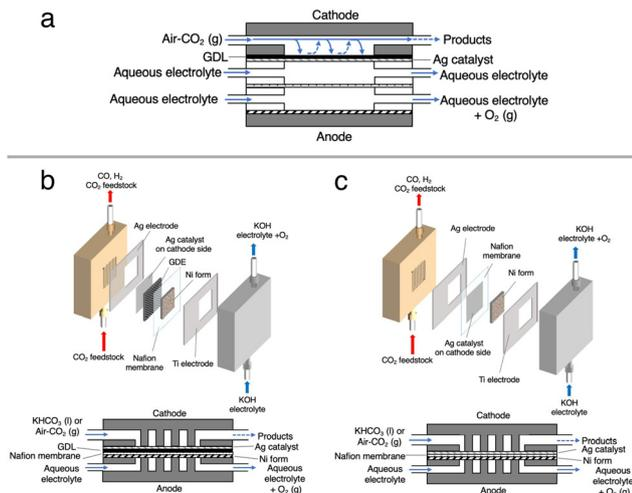
**Fig. 2** Side view of (a) a conventional three-chamber cell, (b) the conventional MEA cell using a carbon based GDE and (c) the Ag MEA-cell. Parts with dots, gray oblique lines and black oblique lines are the membrane, cathode anode catalysts and carbon-based GDE, respectively. System configuration of (b) the conventional MEA-cell using GDE and (c) the Ag MEA-cell.
