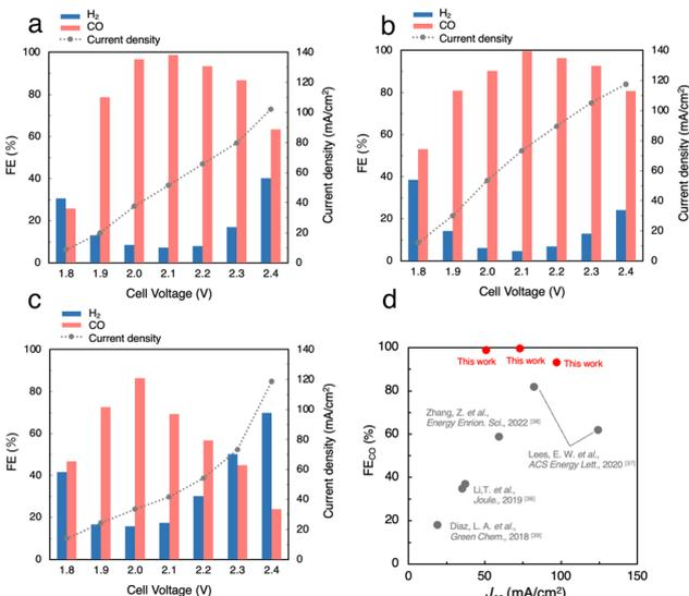
Fig. 4 Faradaic efficiency (FE) and current density (*J*) for the CO<sub>2</sub>RR using (a) 2.0 M BCS and (b) CO<sub>2</sub>-sol and (c) air-CO<sub>2</sub>-sol. (d) Comparison of state-of-the-art performances for the CO<sub>2</sub>RR using BCS coupled with CO<sub>2</sub> capture.
