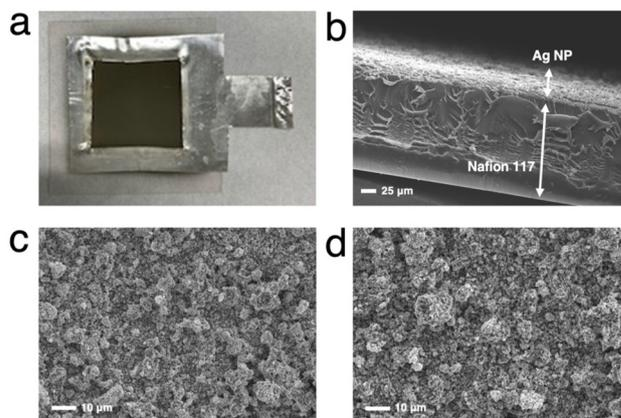
Fig. 3 (a) A photograph of the MEA for the Ag MEA-cell and (b) the cross-section SEM image of the MEA with 2.5 mg cm<sup>-2</sup> of Ag NPs. SEM images of the Ag NPs coated on the MEA (c) before and (d) after the CO<sub>2</sub>RR in BCS.
