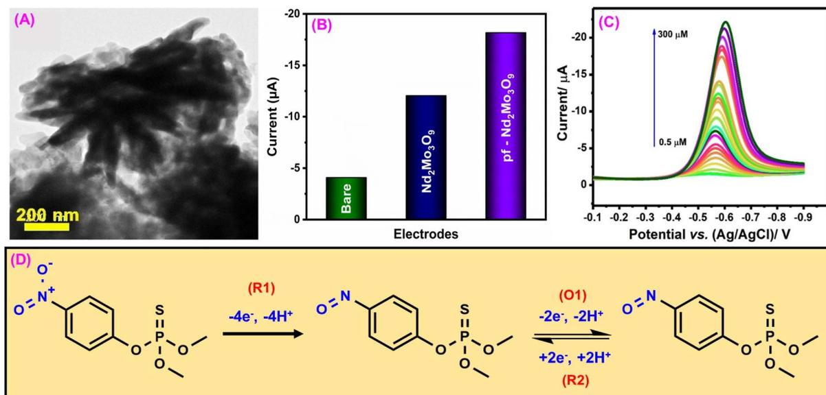
Fig. 2 (A) TEM image of pf- $\text{Nd}_2\text{Mo}_3\text{O}_9$ . (B) CV investigation of the bare GCE (green),  $\text{Nd}_2\text{Mo}_3\text{O}_9$  (blue), and pf- $\text{Nd}_2\text{Mo}_3\text{O}_9$  (purple). (C) DPV signal of pf- $\text{Nd}_2\text{Mo}_3\text{O}_9$  for MPN detection. (D) Electrochemical detection mechanism of MPN<sup>103</sup> (modified). ((A and C) License number: 5542351439158).
