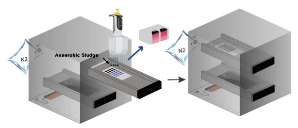
Fig. 1 The design of black box for colorimetric identification on paper-microwell-based and smartphone-assisted analytical device.
