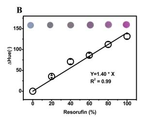
Fig. 3 (A) The effect of sludge sample volume and condensity on speed of color change due to resazurin reduction by anaerobic sludge; (B) the correlation between  $\Delta$ Hue value and resorufin ratio in resorufin/resazurin mixture on Whatman Grade 1 chromatography paper.
