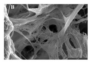
Fig. 2 (A) The anaerobic sludge granular size distribution; (B) the SEM of Whatman Grade 1 chromatography paper.
