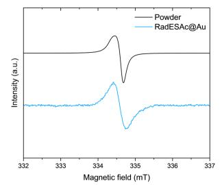
Fig. 2 X-band ( $\nu$  = 9.399030 GHz) EPR spectra acquired on **RadESAc** powder and on the RadESAc@Au monolayer assembled on gold at 30 K.
