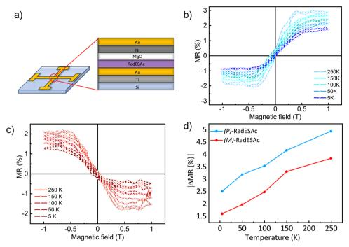
Fig. 4 (a) Scheme of the magnetoresistance device with magnification on the cross junction. Magnetoresistance percentage in the range  $\pm 1$  T of (b) (P)-RadESAc@Au and of (c) (M)-RadESAc@Au monolayers. (d) | \( \Delta MR (%) \)| values as a function of the temperature for both the enantiomers.
