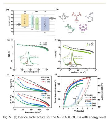
alignment; (b) the chemical structures of the relevant materials used in the device, EQE-luminance curves with EL for (c) BTPCzBN and (d) BTPBN; (e) current efficiency (CE)- and power efficiency (PE)-luminance curves; (f) voltage-luminance-current density curves.
