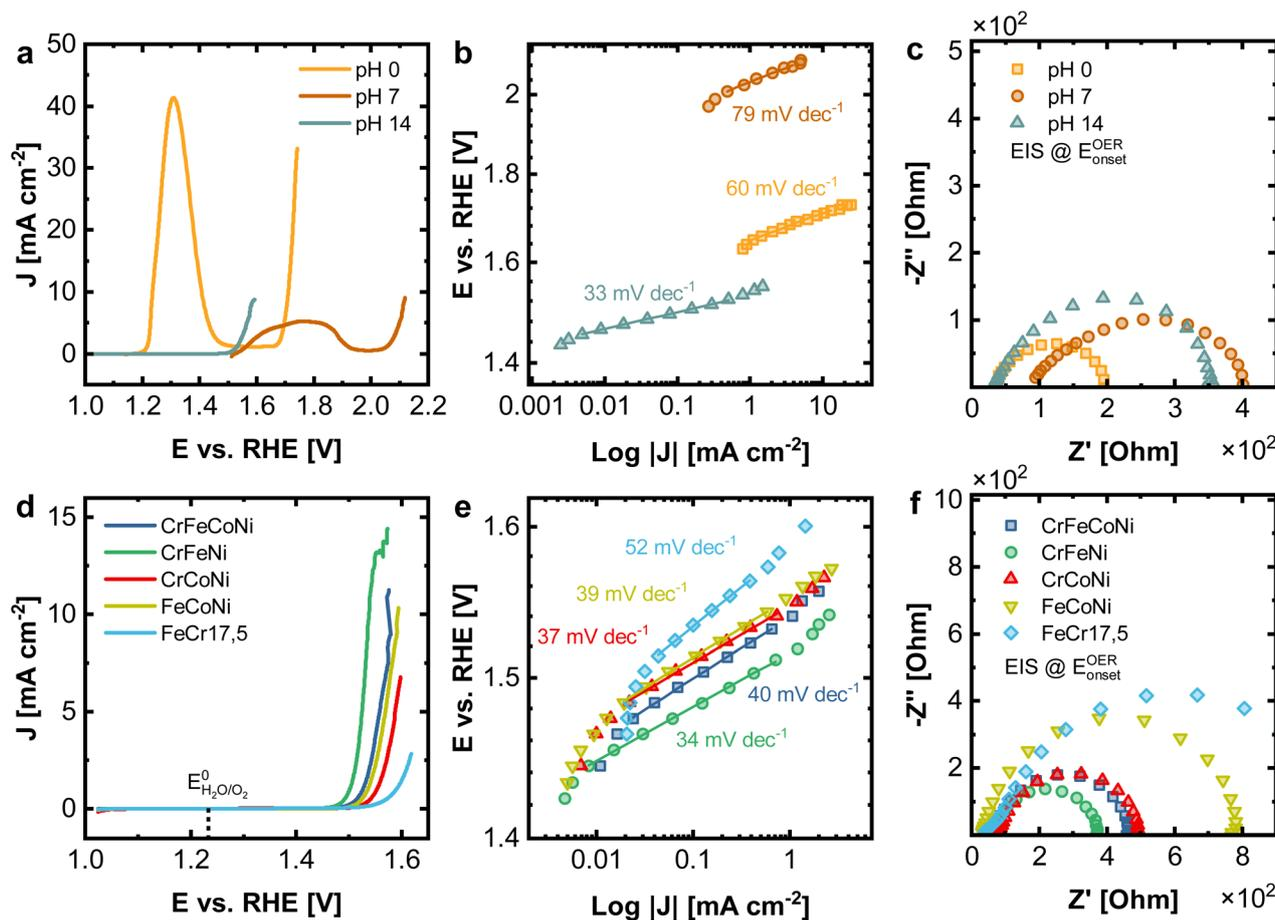
Fig. 5 (a–c) Electrochemical characterization of CrMnFeCoNi under different reaction conditions (1 M H<sub>2</sub>SO<sub>4</sub> (pH 0), 1 M Na<sub>2</sub>SO<sub>4</sub> neutral (pH 7) and 1 M KOH alkaline (pH 14)) as well as (d–f) CrFeCoNi, CrFeNi, CrCoNi, FeCoNi and FeCr17.5 (all 1 M KOH). (a and d) LSV experiments, (b and e) Tafel plots with obtained Tafel slopes, (c and f) EIS spectra performed at the respective OER onset potential.
