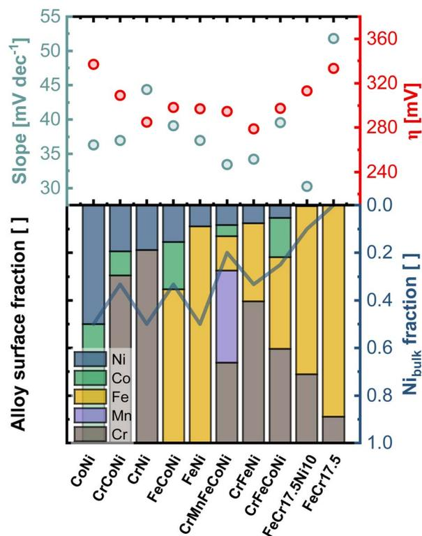
Fig. 6 Comparison of the electrocatalytic activity of all investigated alloys, expressed via the Tafel slope and OER onset-overpotential ( $\eta$ ), and the composition in the first nm of the surface region, with indicated Ni bulk fraction (blue line). Sorted by descending amount of Ni in the outermost layers.
