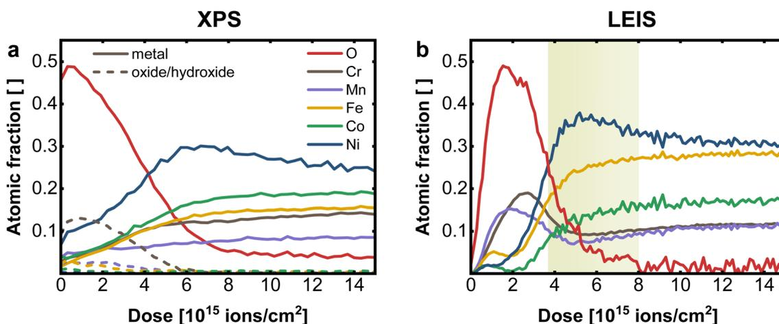
Fig. 3 Comparison of sputter depth profiles on CrMnFeCoNi performed with (a) XPS and (b) LEIS. Depletion zone of Mn and Cr in LEIS is highlighted in yellow. A sputter dose of  $2.19 \times 10^{15}$  ions  $\text{cm}^{-2}$  corresponds to an estimated depth of  $0.6 \pm 0.1$  nm (LEIS) resp.  $0.7 \pm 0.1$  nm (XPS).
