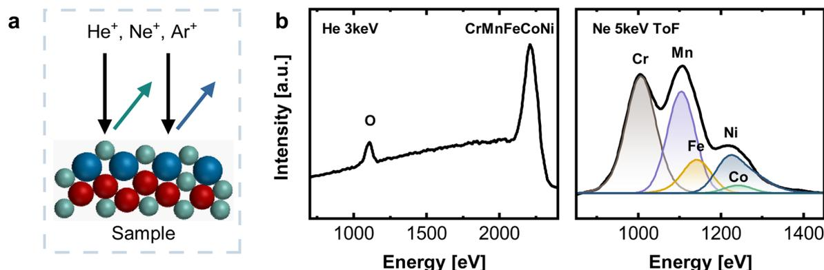
Fig. 2 (a) Working principle of LEIS with indicated pathways of primary (black) and scattered (green, blue) ions. (b) LEIS spectra on the native oxide of CrMnFeCoNi recorded with  $\text{He}^+$  3 keV (left) and  $\text{Ne}^+$  5 keV (right), after a sputter dose of  $2.19 \times 10^{15}$  ions  $\text{cm}^{-2}$ .
