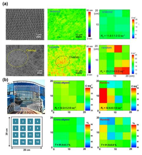
Fig. 5 Comparison of ordered and random Ag NW FTEs. (a) SEM images, AFM height profile, sheet resistance distribution. Reproduced with permission.<sup>101</sup> Copyright 2024, Wiley-VCH. (b) Photograph of large scale (20 × 20 cm<sup>2</sup>) FTE and the mapping showing the distribution of sheet resistance and transmittance for the cross-aligned and random Ag NW FTEs. Reproduced with permission.<sup>102</sup> Copyright 2017, American Chemical Society.
