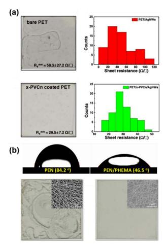
Fig. 8 The substrate treatment or coating for uniform dispersion of metallic nanowires. (a) Optical images and sheet resistance distribution of Ag NW based FTEs on bare PET and the x-PVCn coated PET substrate. Reproduced with permission.<sup>115</sup> Copyright 2020, American Chemical Society. (b) Contact angle and optical images of Ag NW FTEs on PEN and PHEMA coated PEN substrates. Reproduced with permission.<sup>123</sup> Copyright 2022, American Chemical Society.
