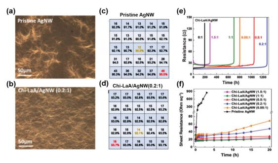
Fig. 3 The stability of the pristine Ag NW and uniform Chi-LaA/Ag NW FTEs. (a and b) Optical images. (c and d) Sheet resistance and transmittance of FTEs with a size of  $6 \times 6 \text{ cm}^2$ . (e) Resistance as a function of time under a current of 250 mA cm<sup>-2</sup>. (f) Sheet resistance as a function of time at high temperature of 180 °C. Reproduced with permission. 71 Copyright 2020, the Royal Society of Chemistry.
