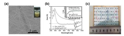
Fig. 2 (a) Well dispersed Ag nano-ink and a SEM image of Ag NW networks. (b) UV-vis curves of haze and transmittance vs. wavelength. (c) Optical image of the Ag NW FTE and its sheet resistance distribution. Reproduced with permission.<sup>64</sup> Copyright 2017, the Royal Society of Chemistry.
