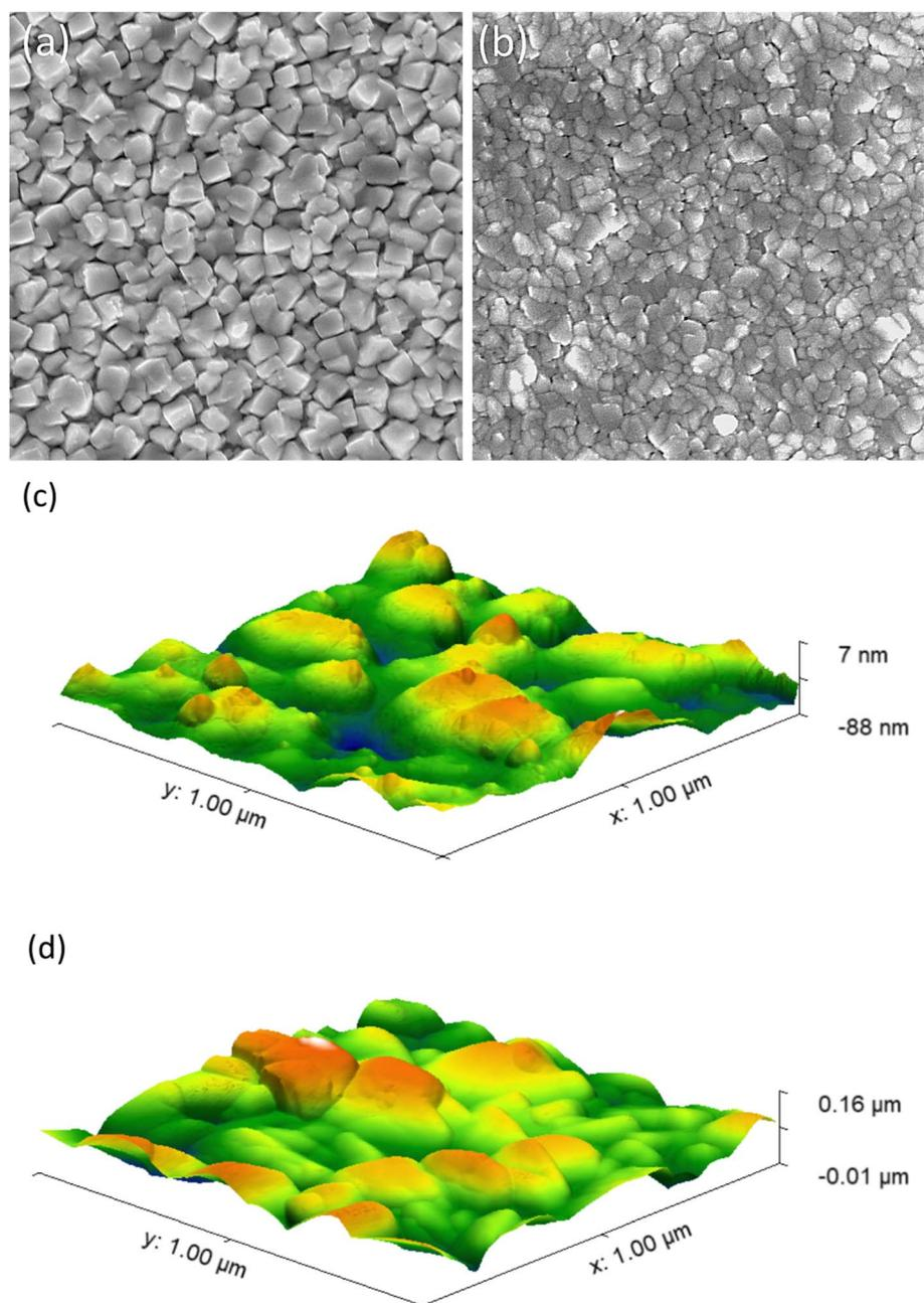
Fig. 4 SEM images of (a)  $\text{BiVO}_4$  and (b) 6% Mo- $\text{BiVO}_4$  taken at 50k magnification [the width of each image represents a distance of  $3.8 \mu\text{m}$ ]. AFM images, of (c)  $\text{BiVO}_4$  and (d) 6% Mo- $\text{BiVO}_4$  measured over a  $1 \mu\text{m} \times 1 \mu\text{m}$  square area.
