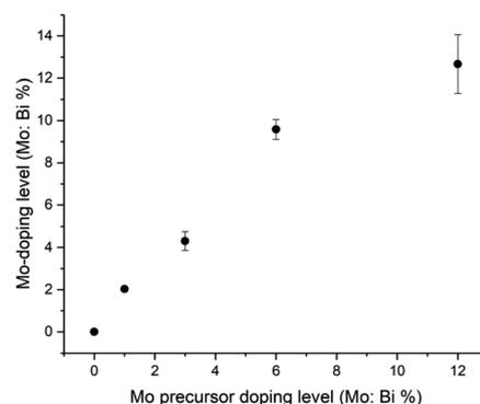
**Fig. 3** A plot of the relationship between Mo precursor dopant level (Mo : V %) vs. the Mo doping level determined by XPS analysis. All values are the average of 3 unique sample locations; with the error bars representing one standard deviation.
