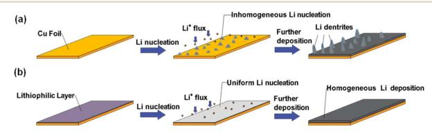
Fig. 8 Schematic diagrams of Li nucleation and growth on (a) bare Cu and (b) Cu with a lithiophilic layer.
