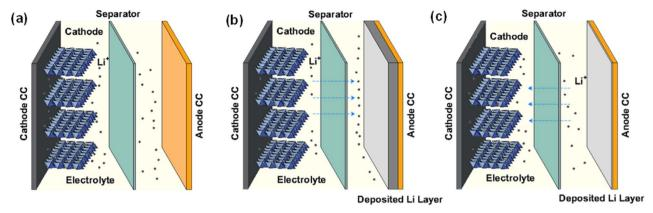
Fig. 1 The basic mechanism of anode-free lithium metal batteries. (a) Schematic of AFLMBs. (b) Charge and (c) discharge processes of AFLMBs.
