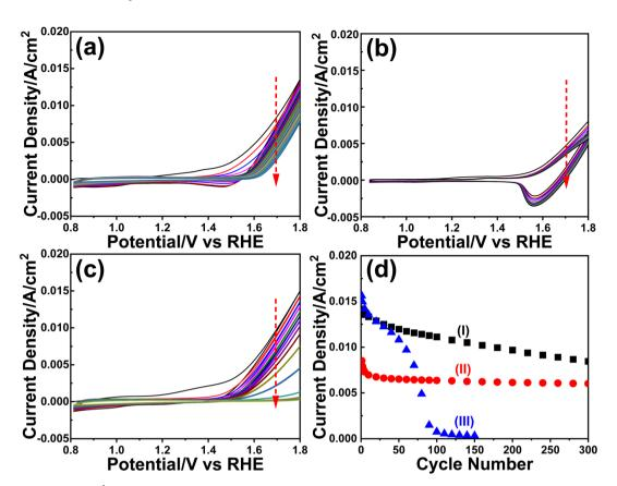
Fig. 6 The CV curves (50 mV s $^{-1}$  scan rate) of the m-LMO-300-F2 electrode in (a) 1.0 M KOH and (b) 1.0 M LiOH and (c) the CV curves (50 mV s $^{-1}$  scan rate) of the m-Mn<sub>3</sub>O<sub>4</sub>-300-F2 electrode in 1.0 M KOH (red arrows indicate the cycling order). (d) Plot of current density values at 1.8 V versus CV cycle numbers of the electrodes, (I) m-LMO-300-F2 in 1.0 M KOH, (II) m-LMO-300-F2 in 1.0 M LiOH, and (III) m-Mn<sub>3</sub>O<sub>4</sub>-300-F2 in 1.0 M KOH.
