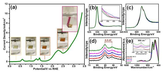
Fig. 4 (a) The LSV curve of the m-LMO-300-F2 electrode between -0.05 and 3.4 V in 1.0 M LiNO $_3$  with a 5 mV s<sup>-1</sup> scan rate (insets: color of the electrodes at indicated potentials) and the XPS spectra of m-LMO-300-F2 at various potentials in the (b) O 1s, (c) Mn 2p, and (d) Mn 3s regions, where black: 1.6 V, red: 1.7 V, blue: 1.8 V, pink: 1.9 V, and green: 2.0 V. (e) The FTIR spectra of m-LMO-300-F2 at various potentials.
