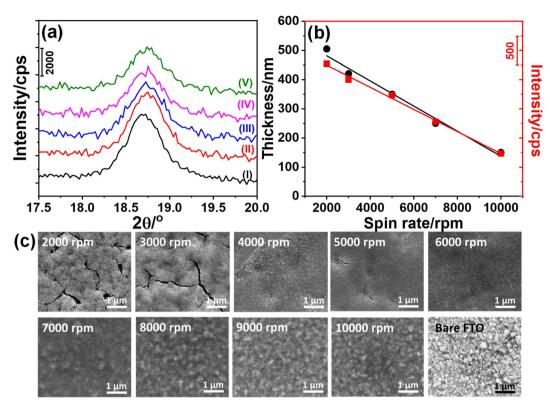
Fig. 1 (a) The XRD patterns of m-LMO-300-F# films between 17.5 and 20.0°, 2 $\theta$ , coated at (I) 2000, (II) 3000, (III) 5000, (IV) 7000 and (V) 10 000 rpm, (b) the plots of the film thickness and X-ray intensity of the m-LMO-300-F# films versus spin-rate (black dots from SEM images and red squares are (111) diffraction line intensity values at 18.7°,  $2\theta$ ), and (c) the SEM images (top view) of the thin films at indicated spin-rates.
