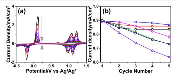
Fig. 3 (a) The CV curves of the m-LMO-300-F2 electrode in 1.0 M LiClO<sub>4</sub> acetonitrile solution (arrows represent the cycle order) and (b) the plot of the current density at 1.4 V of the m-LMO-300-F2 electrode versus cycle numbers in 1.0 M LiNO<sub>3</sub> aqueous solution with respect to the starting potential of a forward sweep in the CV curves, where black: 0.75 V, red: 0.45 V, blue: 0.15 V, pink: 0.05 V, green: -0.05 V, dark blue: -0.15 V, and purple: -0.2 V.
