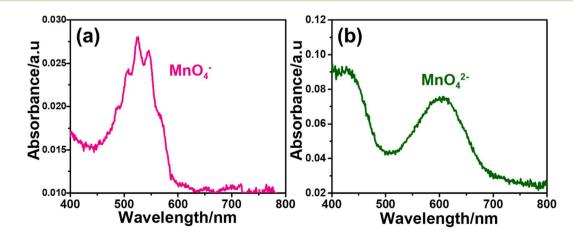
Fig. 7 The visible absorption spectrum of electrolyte during (a)  $MnO_4$  release in acidic media and (b) upon aging the same solution after 20 CV cycles.
