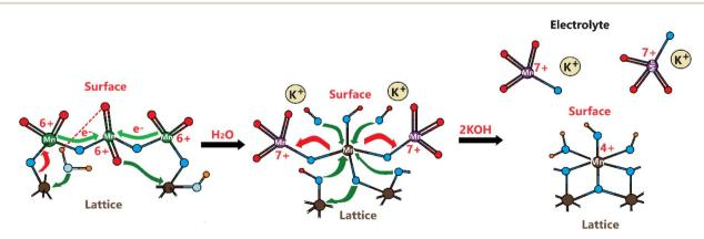
Scheme 1 Electrode degradation mechanism of LiMn<sub>2</sub>O<sub>4</sub> electrodes during the OER.
