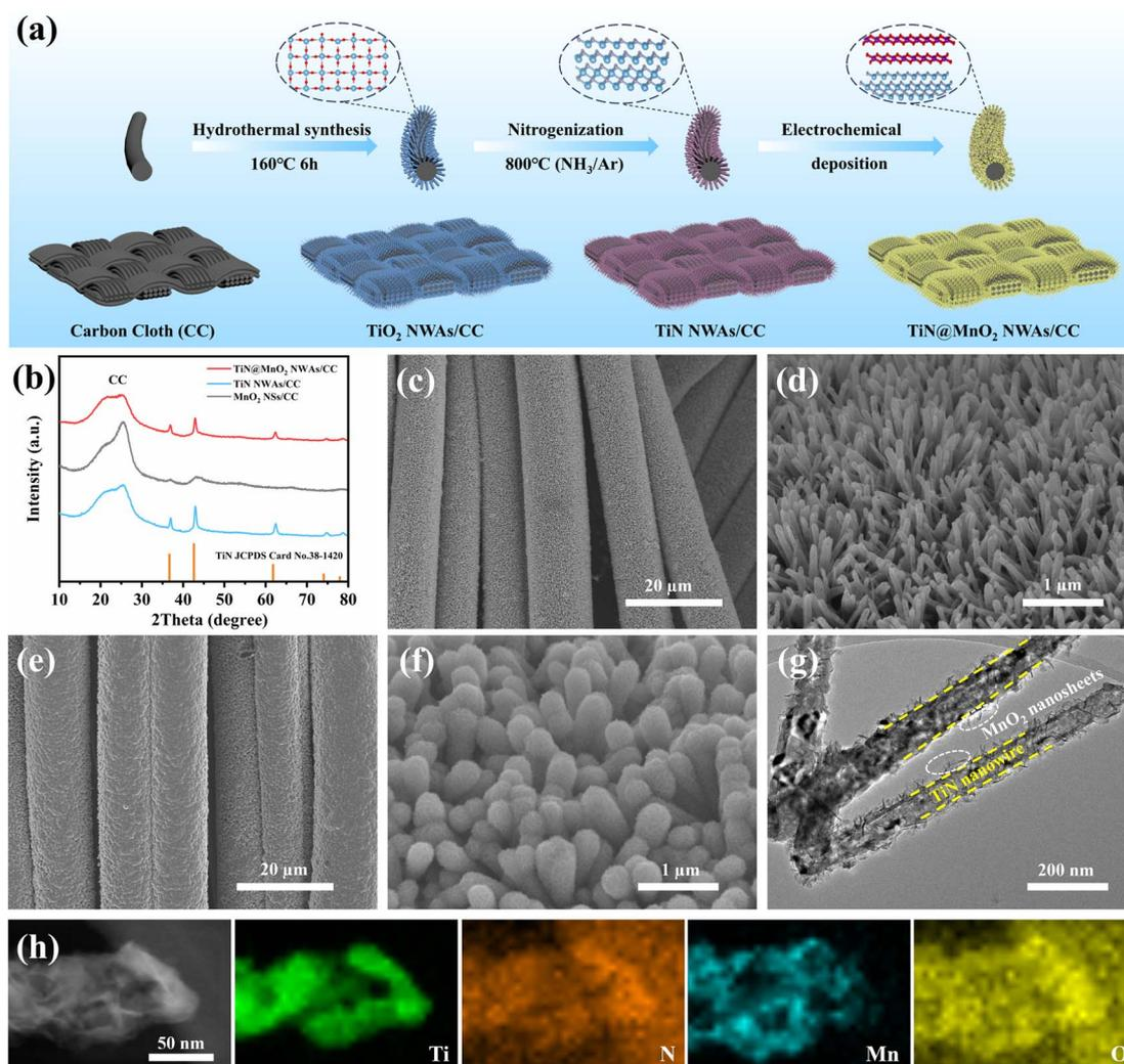
Fig. 2 (a) Schematic diagram of preparation of TiN@MnO<sub>2</sub> NWAs/CC. (b) XRD patterns of TiN@MnO<sub>2</sub> NWAs/CC, TiN NWAs/CC and MnO<sub>2</sub> NSs/CC. SEM images of TiN NWAs/CC (c, d) and TiN@MnO<sub>2</sub> NWAs/CC (e, f) at different magnifications. TEM image (g) and EDS element mapping (h) of single TiN@MnO<sub>2</sub> nanowires.
