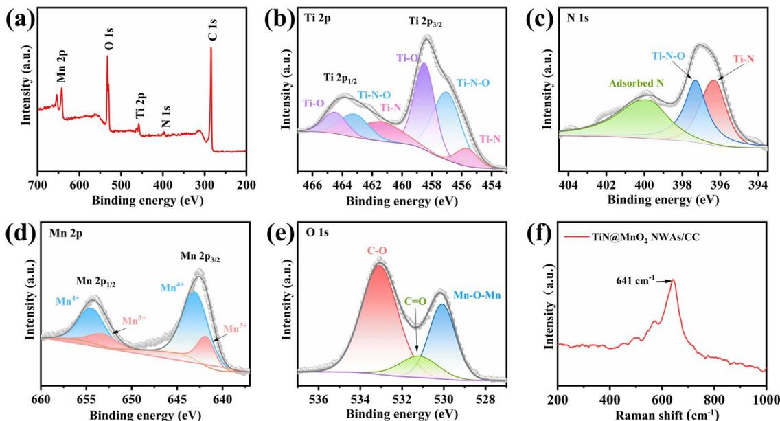
Fig. 3 (a) Full XPS survey spectrum of TiN@MnO<sub>2</sub> NWAs/CC and high-resolution Ti 2p (b), N 1s (c), Mn 2p (d), and O 1s (e) XPS spectra. (f) Raman spectrum of TiN@MnO<sub>2</sub> NWAs/CC.
