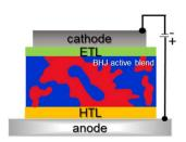
Fig. 9 Schematic representation of a Bulk Heterojunction (BHJ) solar cell.
