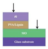
Fig. 8 Vertical sandwich structure of Mo/lignin and PVA film/AI. Adapted from W. Zhang et al. (2023).65 Copyright 2023, IEE.
