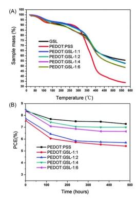
Fig. 10 (A) Thermogravimetric analyses (TGA) of GSL polymer, PEDOT: PSS and PEDOT: GSLs. (B) Lifetime tests of the solar cells based on PEDOT: PSS and PEDOT: GSLs as HTLs, respectively. Reproduced from N. Hong *et al.* (2016).<sup>66</sup> Copyright 2016, Royal Society of Chemistry.
